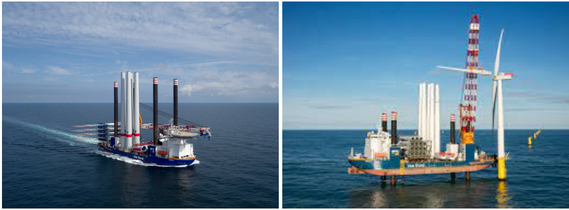
Figure 2.1: Transport to installation side by jack-up vessel Aeolus of Van Oord.
