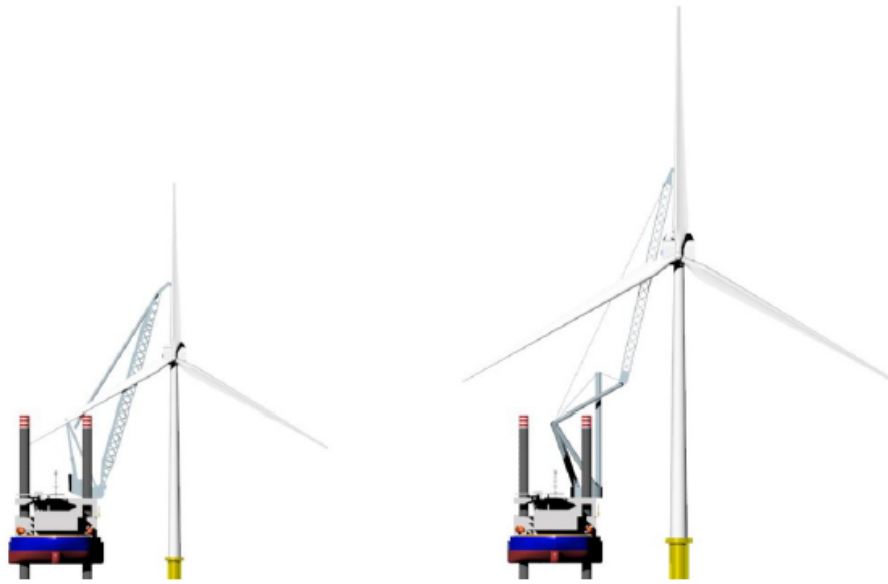
Figure 1.1: Comparison of the lifting height of a luffing boom crane with the lifting height of a Tetrahedron crane.
