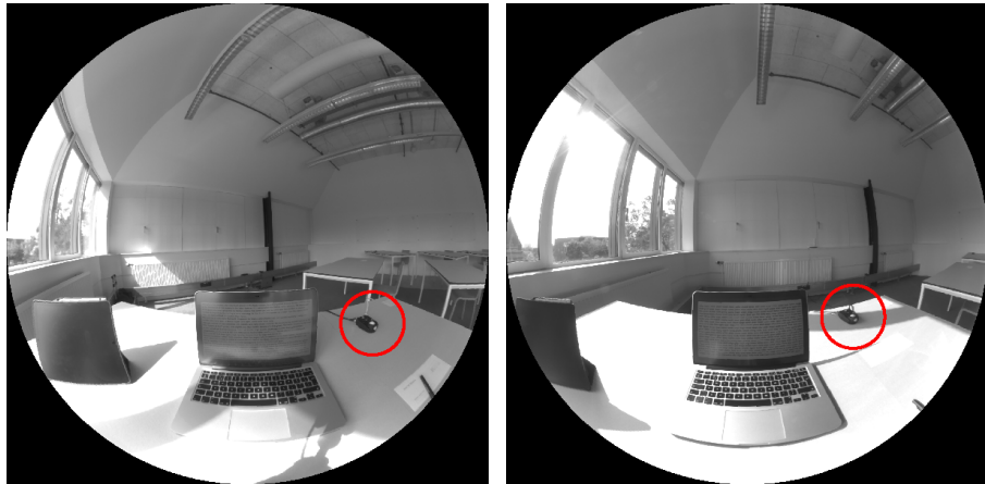
FIG. 4.12 Variation of light between the sitting position and the point of illuminance measurement. Illuminance meter is circled in red.
