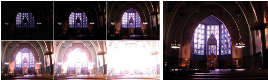
FIG. 3.4 Sequence of low dynamic range photographs captured with different exposures (aperture fixed at F2.6, ISO 100, shutter speed range 1/60" - 15") and the resulting high dynamic range image. Source: (Jacobs, 2007).
