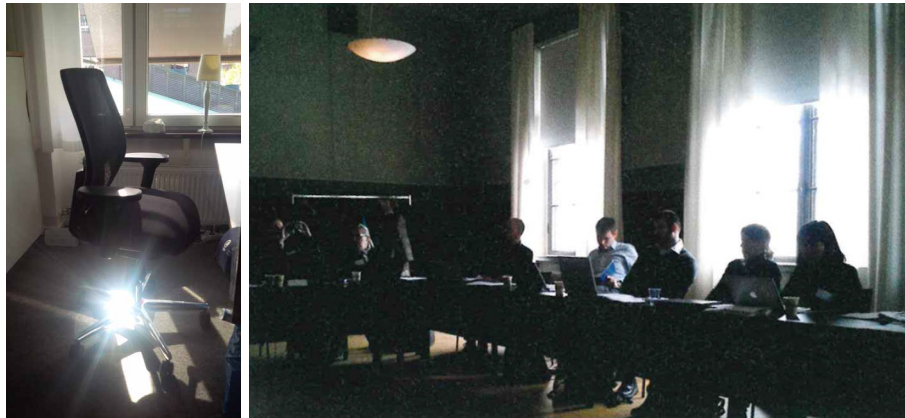
FIG. 1.1 A situation that can result in disability glare (left) (source: by the author) and a situation that can result in discomfort glare (right) (source: Dubois et al., 2019). In the left image, the extreme brightness of the reflected light patch can impair seeing for an observer looking in the direction of the window. On the right image, the very bright windows in the direct view of the observer in this meeting room, creates visual discomfort.
