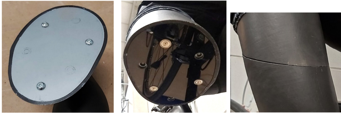
Figure 4: The magnetic interface in the upper leg portion. A similar interface was introduced for the upper body.
