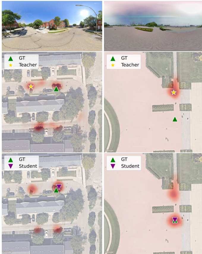
Figure 6.4: CCVPE teacher and student model’s predictions on VIGOR test set. The red color denotes the localization probability (a darker color means a higher probability).
