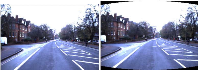
Figure 4.15: An example ground image from Oxford RobotCar dataset. Left: perspective projection (no image processing was applied). Right: equirectangular projection (pre-processed image).
