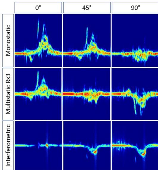
**FIGURE 5** Simulated radar returns for action (II): (a) mD signatures from the mono radar at aspect angles  $0^\circ$ ,  $45^\circ$  and  $90^\circ$ ; (b) simulated mD signatures from the multistatic radar at receiver 3 (bistatic angle  $90^\circ$ ) at aspect angle  $0^\circ$ ,  $45^\circ$  and  $90^\circ$  and (c) frequency responses from the interferometric radar channel with a 10-m baseline at  $0^\circ$ ,  $45^\circ$  and  $90^\circ$
