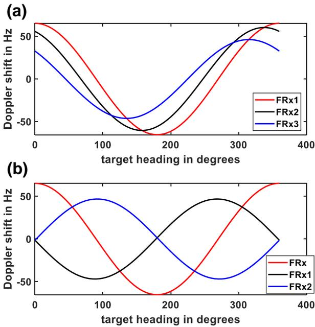
**FIGURE 3** The expected Doppler shifts for: (a) the CM configuration with nodes at 0°, 45° and 90° and (b) the in-line configuration with a 10 m baseline (Rx<sub>1</sub>/Rx<sub>2</sub> have the same Doppler shifts in the interferometric case) for a carrier frequency of 9.8 GHz
