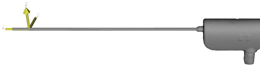
Figure 4.4: Origin of STL file ablation needle placed at the center of the ablating area on the antenna.
