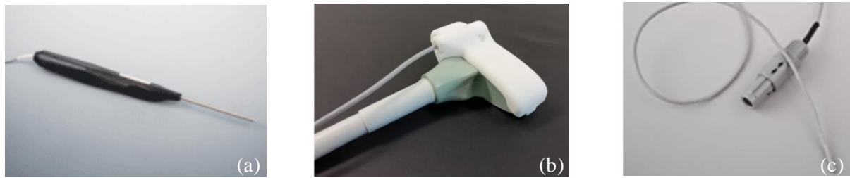
Figure 1.7: Tracked instruments surgical liver navigation workflow: (a) the Aurora 6DOF Probe, (b) the custom-made adapter for BK US probe, and (c) the Aurora 6DOF Cable Tool used for attachment to the liver surface.
