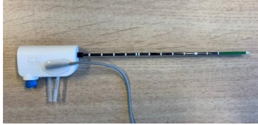
Figure 3.7: Sensor attached onto shaft of the ablation needle.
