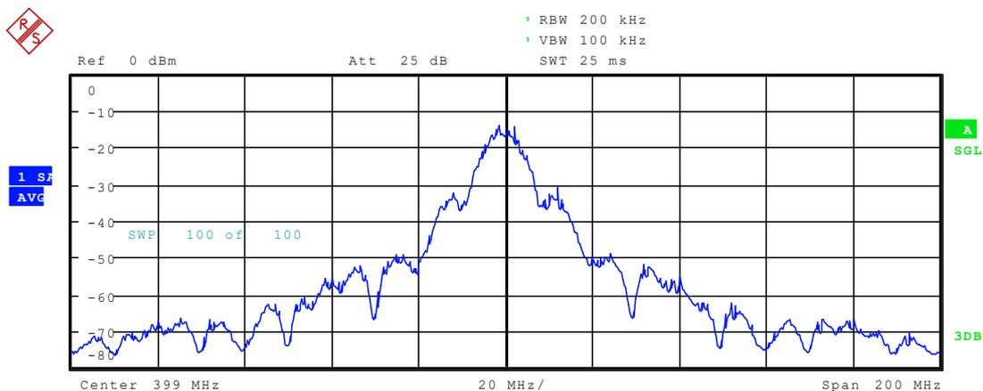
Figure 4.23: Measured spectrum of the RF output clock modulated with a 60 Mb/s (10 MSymbol/s) 64-PSK signal at the RF channel frequency of  $3188 \div 8$  MHz.
