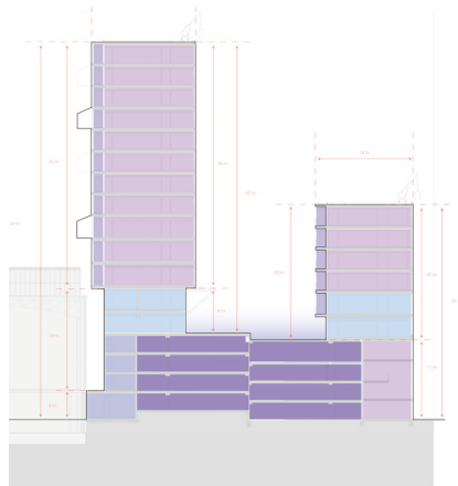
Figure 178: Accessibility and functions Section Schiecentrale. (Machgeels, D., 2020) Analysed from Section (Mei architects and planners, 2020)
