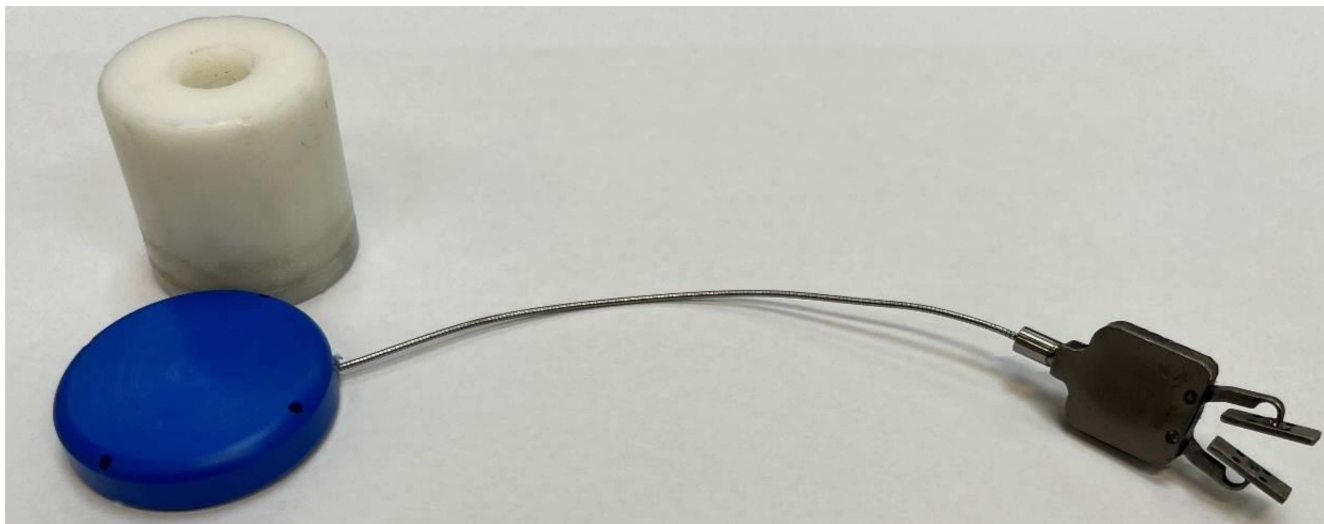
Fig. 10. Manufactured prototype of the implant device used in the experimental setup, and the external magnets that can be utilized to actuate the prototype.
