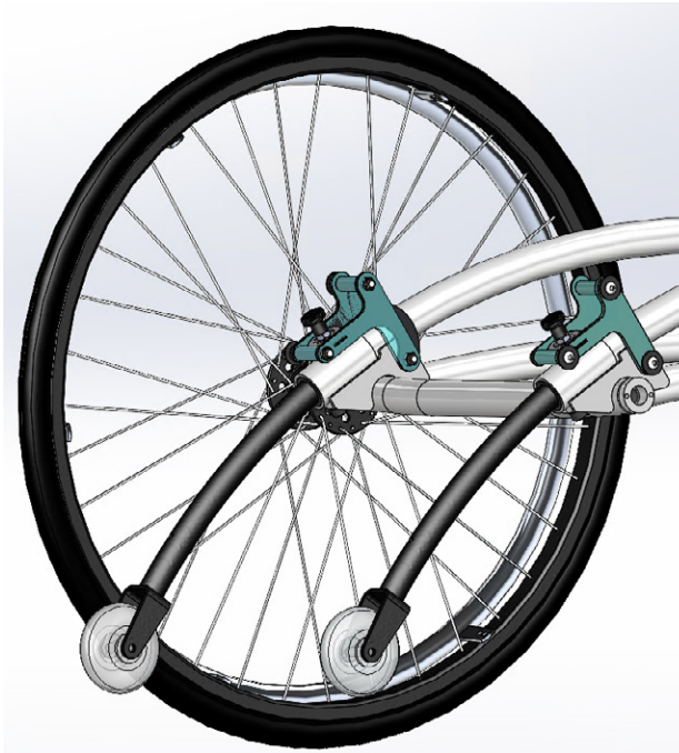
Figure 22, Current fender bracket, left & right specific
