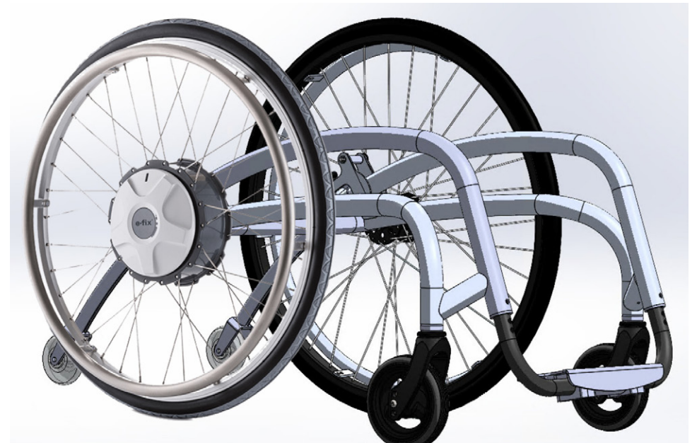
Figure 36, Common electric wheel on the frame
