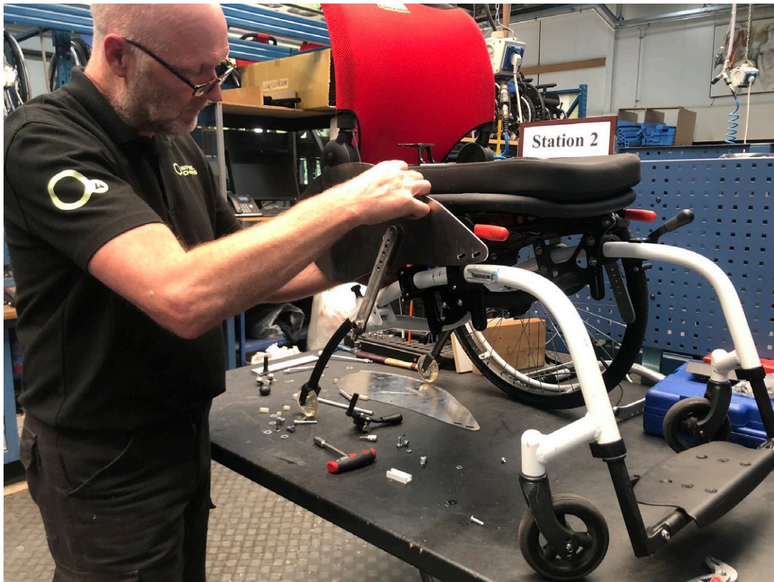
Figure 46, Assembly worker building the new fender assembly at O4
