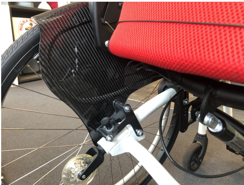
Figure 20, Add-on to the frame, not integrated
