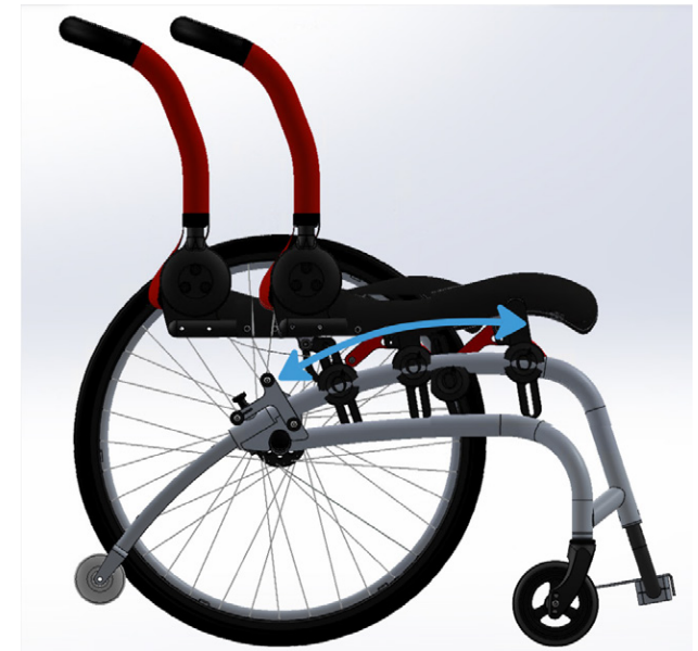
Figure 11, Adjustability of seat activity (front & back position, over curved tube, seat height changes with it
