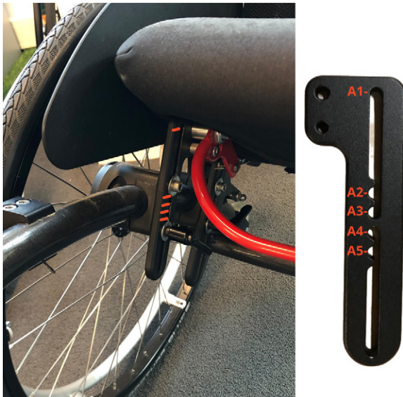
Figure 24, Seat height bracket with indications
