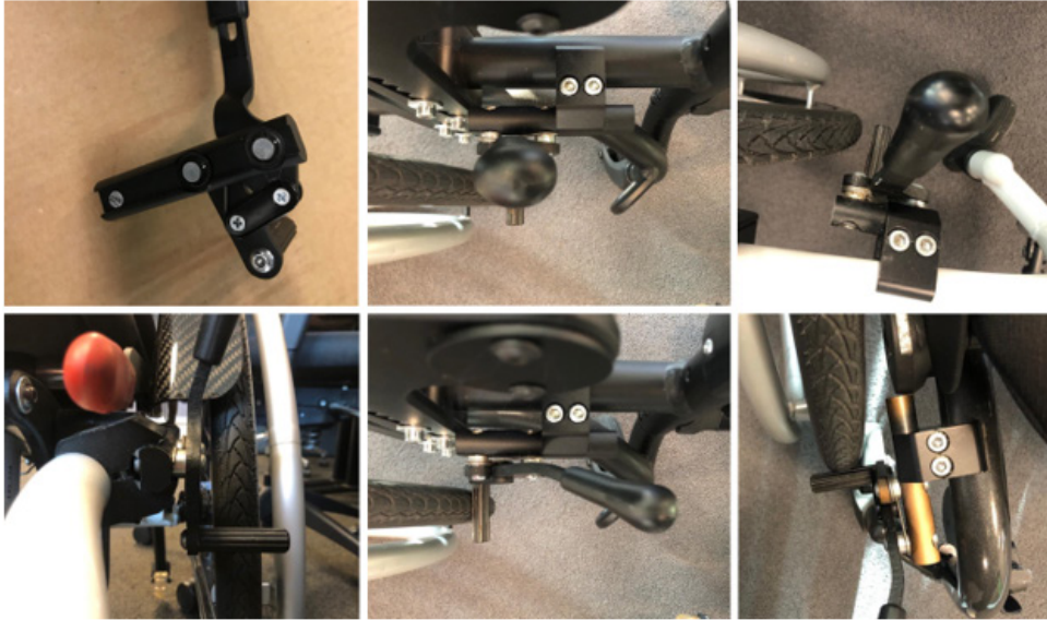
Figure 11, Attachment of the brake. Note how the brake itself can rotate in the clamp, and the clamp can turn on the frame tube.
