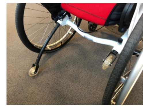
Figure 9, the anti-tip prevention tubes, at the back of the wheelchair
