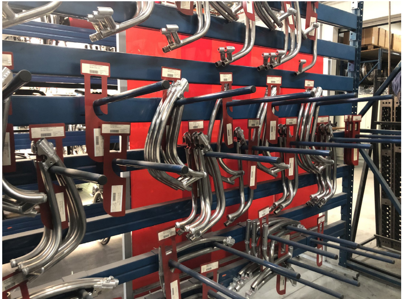
Figure 9, Pre-welded sub-assembly stock at O4
