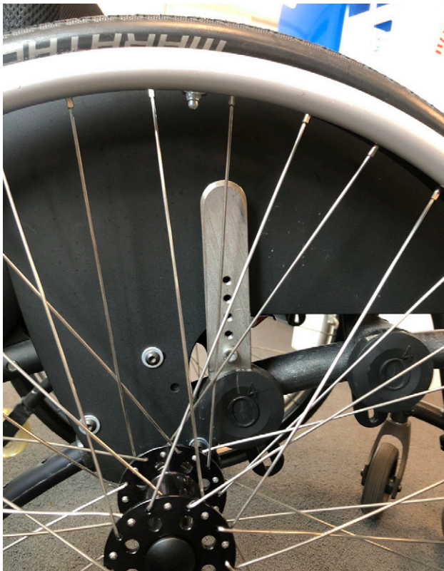
Figure 34, Current E-wheel fixation bracket
