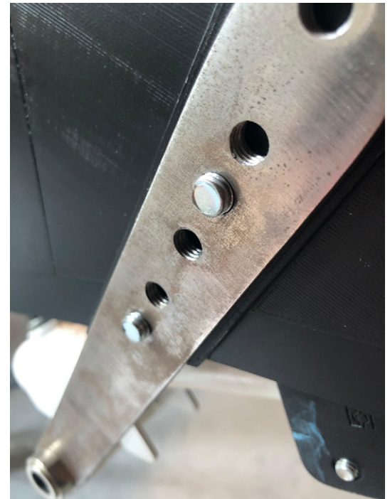
Figure 52, Threaded holes in the axle bracket
