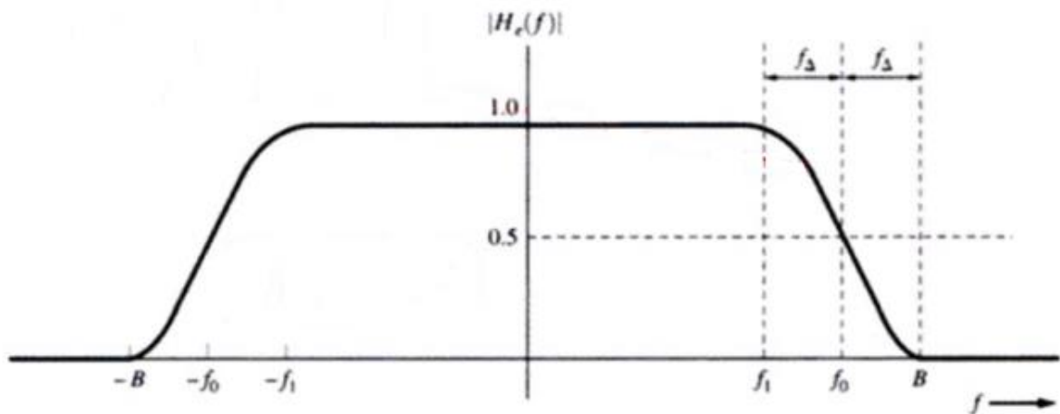
Figure 4.2: Schematic band-pass signal of a root raised cosine filter [8]
