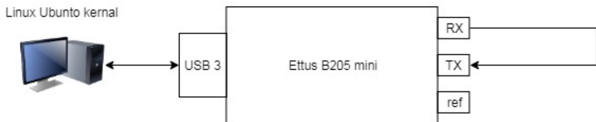
Figure 4.5: Ettus loop back schematic
