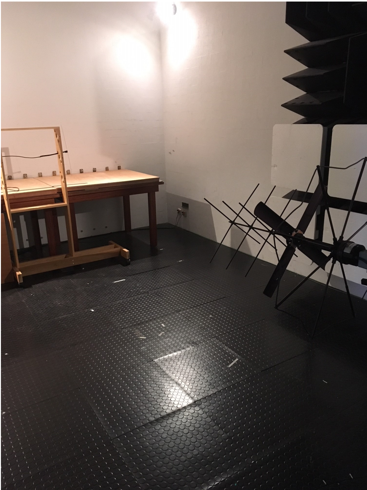
Figure C.2: Measurement Setup in configuration 3 (reflector and one set of directors)
