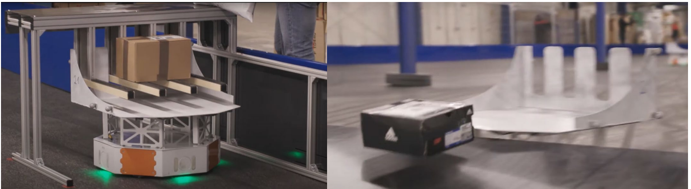
Figure 14- Load Runner Picking and Placement Image Source: https://www.youtube.com/watch?v=XtDjhCBFe7Y
