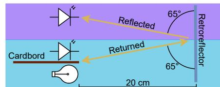
Fig. 2: The evaluation setup used to test (retro)reflectors.
