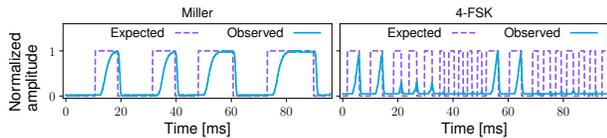
Fig. 6: Default Miller and 4-FSK encoded messages.
