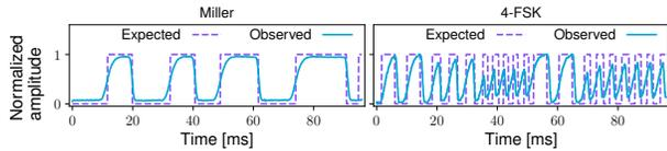
Fig. 7: Enhanced Miller and 4-FSK encoded messages.
