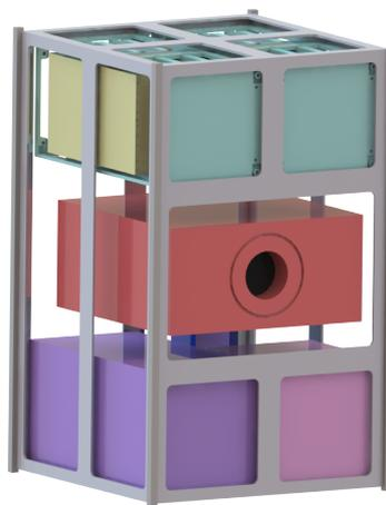
**Figure 4.18:** Spacecraft as seen from the back showing the modified back panel and the propulsion system thruster.
