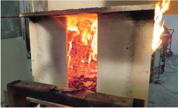
Figure 10: Compartment 2.2 with three CLT walls remained in flaming combustion after the initial fire was stopped due to fall-off of delaminated layers.
