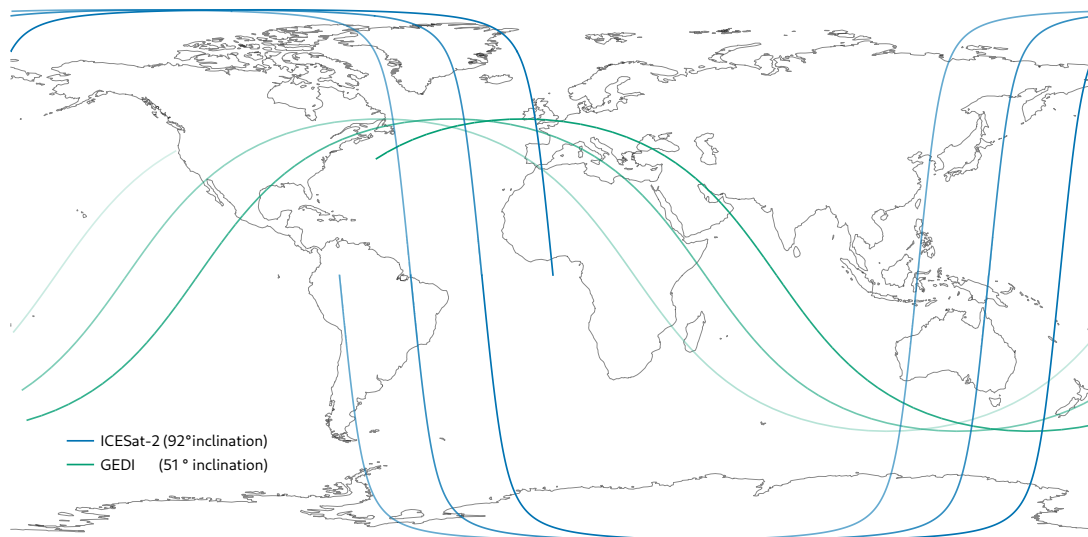
Figure 2.1.: Orbit illustration of two space-borne LiDAR Source:Pronk et al. [2022]
