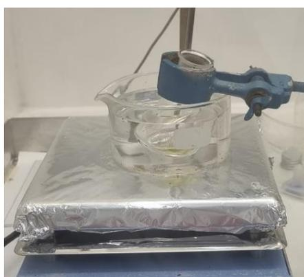
**Figure 7.** Set-up for the synthesis of ferric sulphate where the Erlenmeyer is placed into an oil bath. A thermometer was placed in the oil bath to monitor the temperature.
