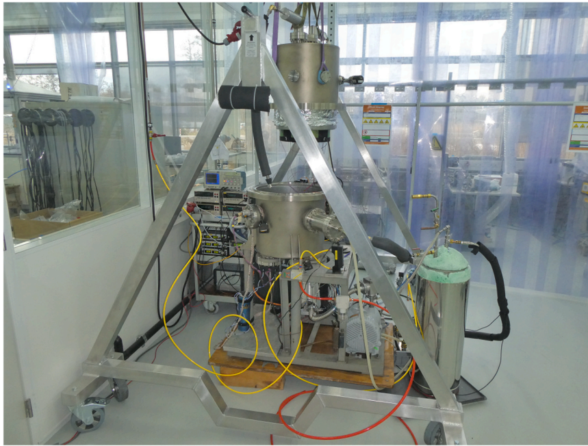
Fig. 4. Open vacuum chamber and control and measurement equipment.
