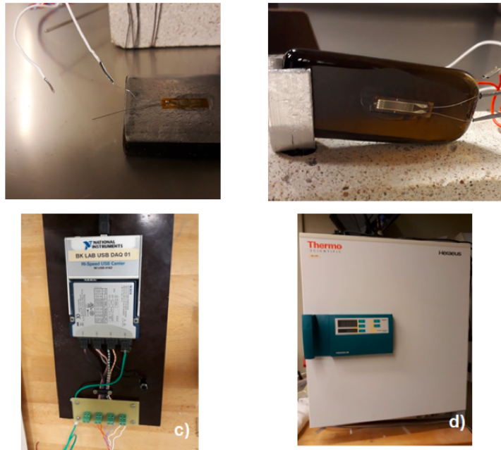
Figure 5.2: The setup a) connexion between wire and gauge b) connexion wire and gauge c) DAQ device d) furnace Heraeus.
