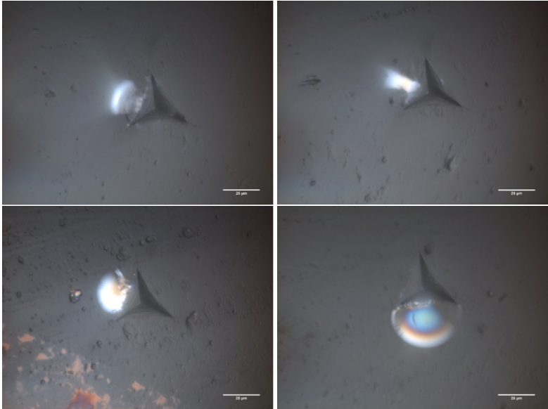
Figure E.22: Four indents of the sample 75\text{KPO}_3\text{-}12.5\text{slag-}12.5\text{Al}_2\text{O}_3 under 2.N analysed by reflected light.
