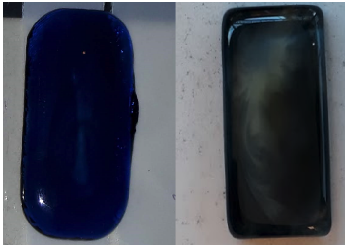
Figure 4.26: The sample 50\text{KPO}_3\text{-}20\text{B}_2\text{O}_3\text{-}15\text{Slag-}15\text{Al}_2\text{O}_3 melted at 1150^\circ\text{C} , and 1250^\circ\text{C} .
