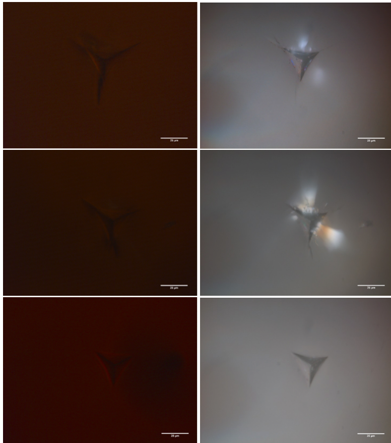
Figure E.32: Three indents of the sample 60KPO 3 -20slag-20Al 2 O 3 under 2N, analysed by transmitted (left) and reflected light (right).
