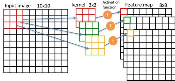
**Figure 2-8:** Convolution of an input image (10x10 pixels) with 3 kernels (3x3 pixels) shown in red, green and yellow, resulting in 3 feature maps (8x8 pixels) that contain the output activation's for a given kernel
