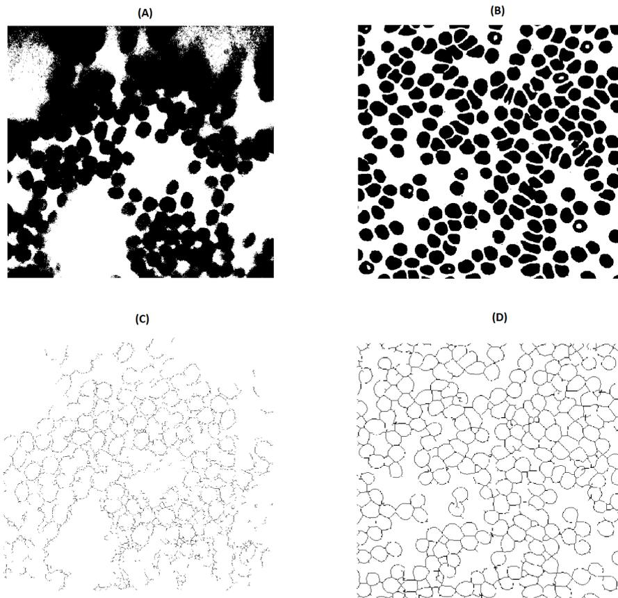
**Figure 2-3:** (A) Smartphone based microscope example image with Otsu's thresholding method. (B) Example image from a light microscope taken from the Mamic Database with Otsu's thresholding method. (C) Smartphone based microscope example image processed with Sio's edge detection algorithm. (D) Example image from a light microscope taken from the Mamic Database processed with Sio's edge detection algorithm.
