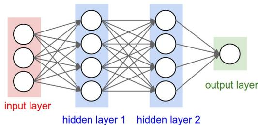
**Figure 2-7:** Example of a 3-layer feed-forward Neural Network (Input layer of 3 neurons, 2 hidden layers with 4 neurons each and an output layer with 2 neurons)
