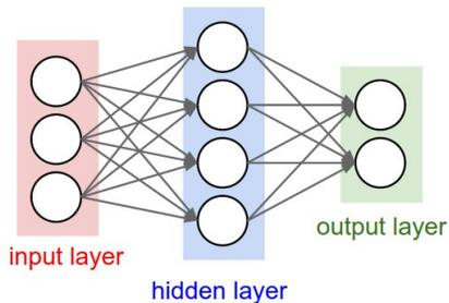
**Figure 2-6:** Example of a 2-layer feed-forward Neural Network (Input layer of 3 neurons, hidden layer with 4 neurons and an output layer with 2 neurons)
