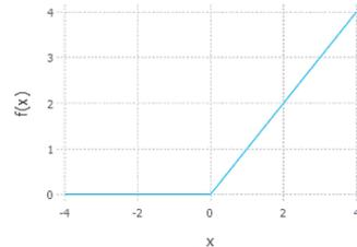
**Figure 2-5:** Rectified Linear Unit (ReLU) activation function , which is zero when  $x < 0$  and then linear with slope 1 when  $x > 0$
