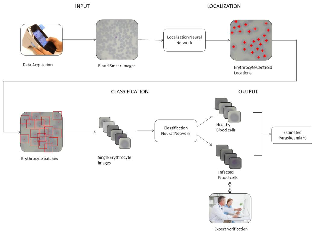
**Figure 3-1:** Overview of the proposed automated diagnostic method for the smartphone based microscope
