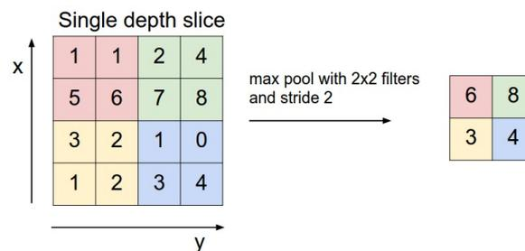
**Figure 2-10:** Max Pooling Layer on a 4x4 input (left) with a 2x2 filter with stride 2, resulting in an output image (right) that is down-sampled by a factor 2 and holds only the maximum values of the coloured areas in the input image
