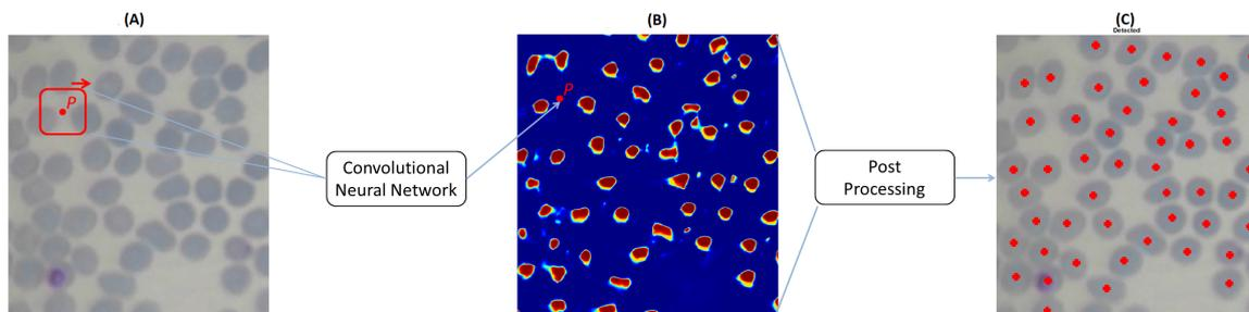
**Figure 3-2:** Localization process, (A) is a part of the input image, where  $p$  depicts the centre of the  $n$  by  $n$  window to be classified as erythrocyte or non-erythrocyte, (B) shows the confidence matrix  $M$  that holds output scores for one output class, (C) shows the centre locations found after post-processing the matrix  $M$
