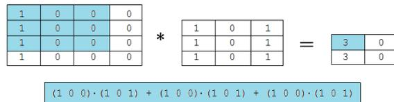
**Figure 2-9:** Convolution equation example, the input image (4x4 pixels) is shown in the left top corner, the kernel (3x3 pixels) in the middle and the output (2x2) pixels in the right top corner, the blue box at the bottom is one the 4 convolutions done, represented in blue in the top images
