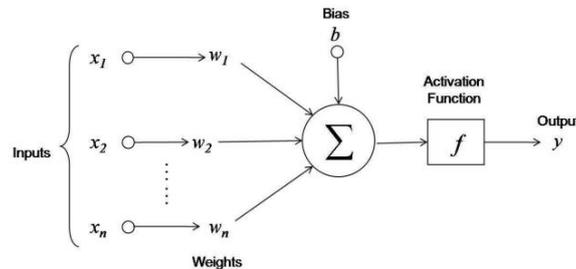
Figure 2-4: Visual representation of the model of a single Artificial Neuron
