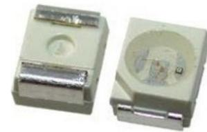
(b) The GUVB-S11SD UVB photodiode by Roithner Lasertechnik, its dimensions are (lxwxh): 3.5 x 2.8 x 1.9 mm [22].
