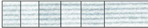
Figure 2.9: Six SE images of line patterns stitched together. A pattern was defined of five horizontal parallel single-pixel wide lines at a mutual distance of 30 nm. The patterning strategy is such that the lines were written serially, ie, one after the other, and from bottom to top. The total dose was 5000 \text{ C/m}^2 . The six patterns, from left to right, were written with 1, 2, 10, 40, 200, and 800 passes, and dwell times of 200, 100, 20, 5, 1, and 0.25 \mu\text{s} , respectively. The contrast of the images was enhanced for clarity, but was performed identically for all the images to maintain the original intensity differences between them.
