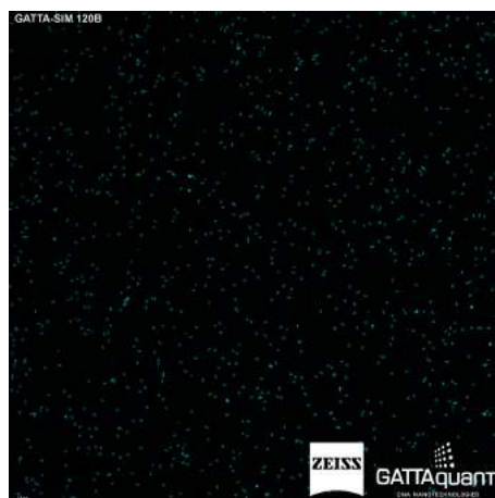
Figure A.1: Superresolution image of Gatta SIM-120B Nanoruler showing randomly oriented folded DNA origami structures tagged with pairs of fluorescent dye molecules (Alexa Fluor 488) at a distance of 120 nm. Image taken from www.gattaquant.com
