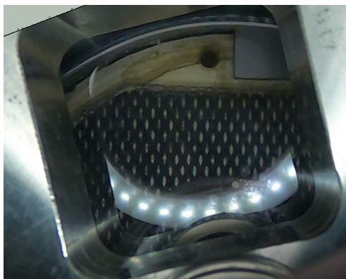
Figure 3.6: GoPro Hero Black 8 overview through the top window in the end plate, onto the top of the electrode and the top channel of the electrolyser cell. The reflection of the lighting in the Bunker Twin is visible in the figure as a the white semicircle.
