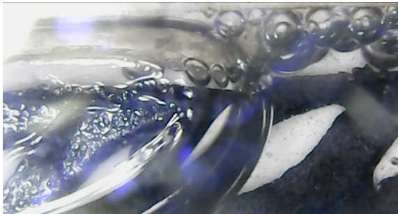
Figure 4.36: Gas liquid interface shifting to the right, due to the increase of volume of oxygen gas in the electrolyser cell due to flow stagnation occurring at the entrance of the top channel.
