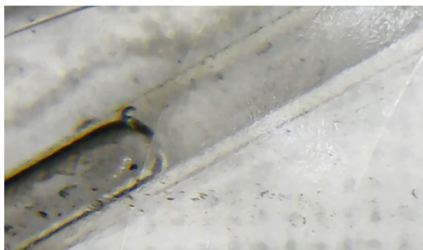
Figure 4.15: Oxygen slug being stuck in the top channel for a pressure range of 47-50 bar.
