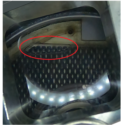
Figure 4.41: Increase of oxygen volume in the electrolyser cell due to oxygen flow stagnation through the channel. The increase in oxygen volume is encircled with the red oval.
