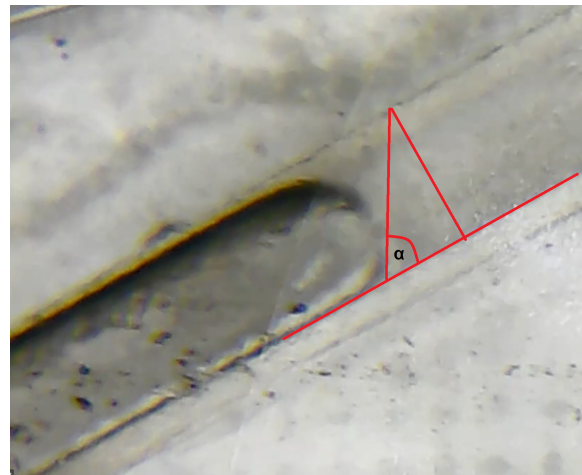
Figure 4.45: Calculation of the contact angle of the slug against the wall the moment the slug starts flowing into the channel completely. The microscope camera is placed at a small angle during these experiments, due to the size of the look through windows, which affects the determining of the contact angle of the slug with the wall.
