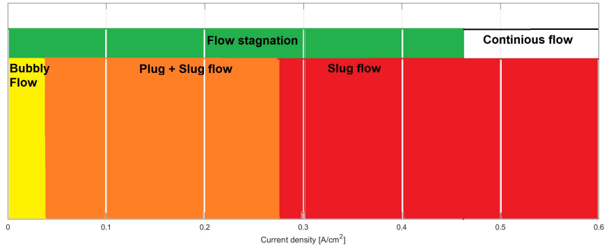
Figure 4.74: ZEF electrolysis system flow characterisation map. The map shows for which current densities flow stagnation occurs,
