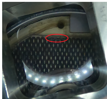
Figure 4.39: Three larges bubbles moving from the right corner of the electrolyser cell towards the entrance of the channel. The bubbles have grown in size due to coalescing with other bubbles stuck a the ceiling of flow upwards to the ceiling. The bubbles are encircled with the red oval.
