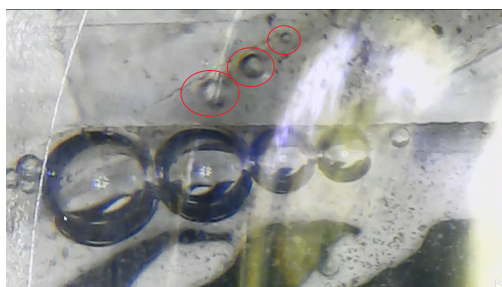
Figure 4.31: Top entrance of the channel when operating at a low current density of 0.017 \text{ A/cm}^2 . Smaller bubbles can be seen entering the channel, encircled in red, even though larger bubbles partially block the channel.
