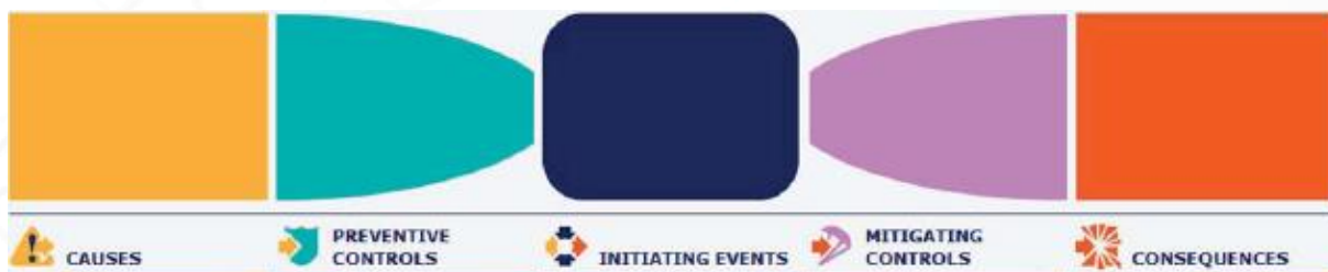
Figure 11 Graphic presentation of the scenario-based BowTie diagram. Retrieved from Harris et al. (2012)
