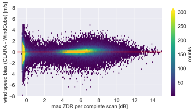
Figure 7. Two-dimensional histograms of the difference between WindCube's and CLARA's wind speed from the lowest 2 km as a function of the maximum ZDR. Note that only data with I_{inv} smaller than 50 % are used.
