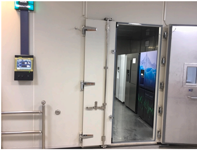
Fig. 5. Walk-in type test room to ensure controlled and constant ambient conditions during experiments.
