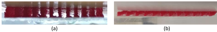
Figure 7.2. Deformation of the 3D CAD model d00102 with the smallest pillar thickness d_1 , under various normal load: (a) 3N and (b) 15 N.
