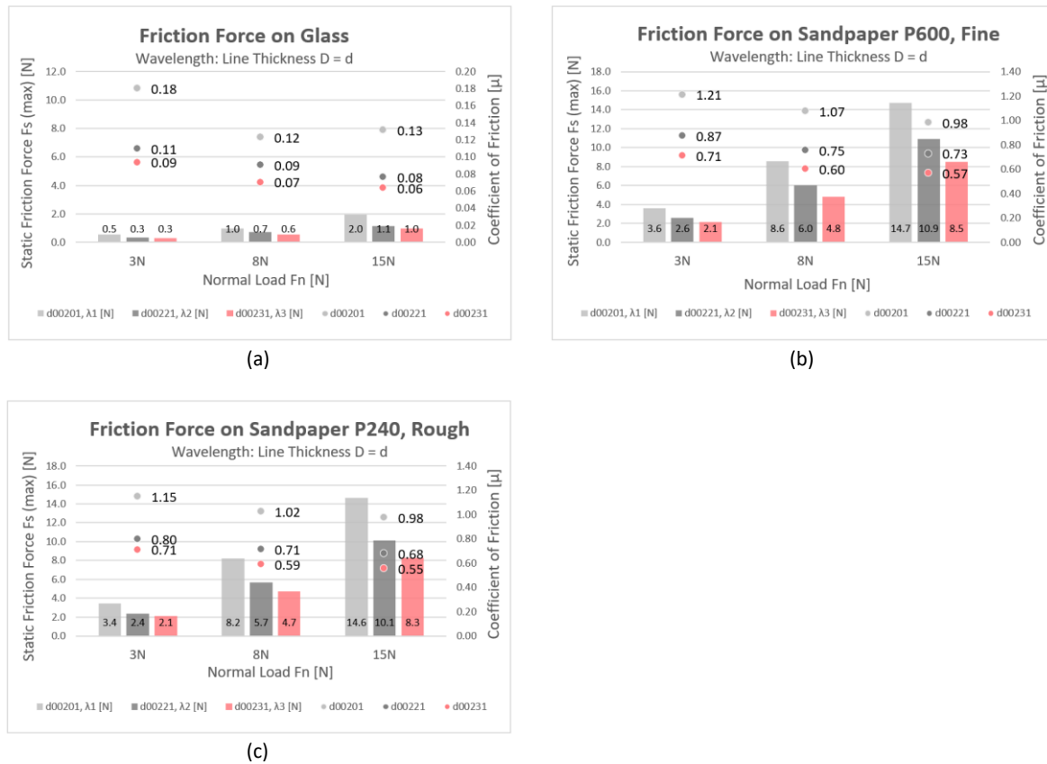
Figure 7.6. The maximum friction force (max.) F_s [N] and coefficient of static friction \mu_s of 3D printed lines, with variable wavelength \lambda_1 = 2.8 mm, \lambda_2 = 1.8 mm and \lambda_3 = 0.8 mm with a correction value that disregards the effects of the number of printed features per \text{mm}^2 out, for the countersurface glass (smooth), sandpaper P600 (fine), and sandpaper P240 (rough). The measured F_s (max) is represented by columns and the corresponding \mu_s is represented by dots.
