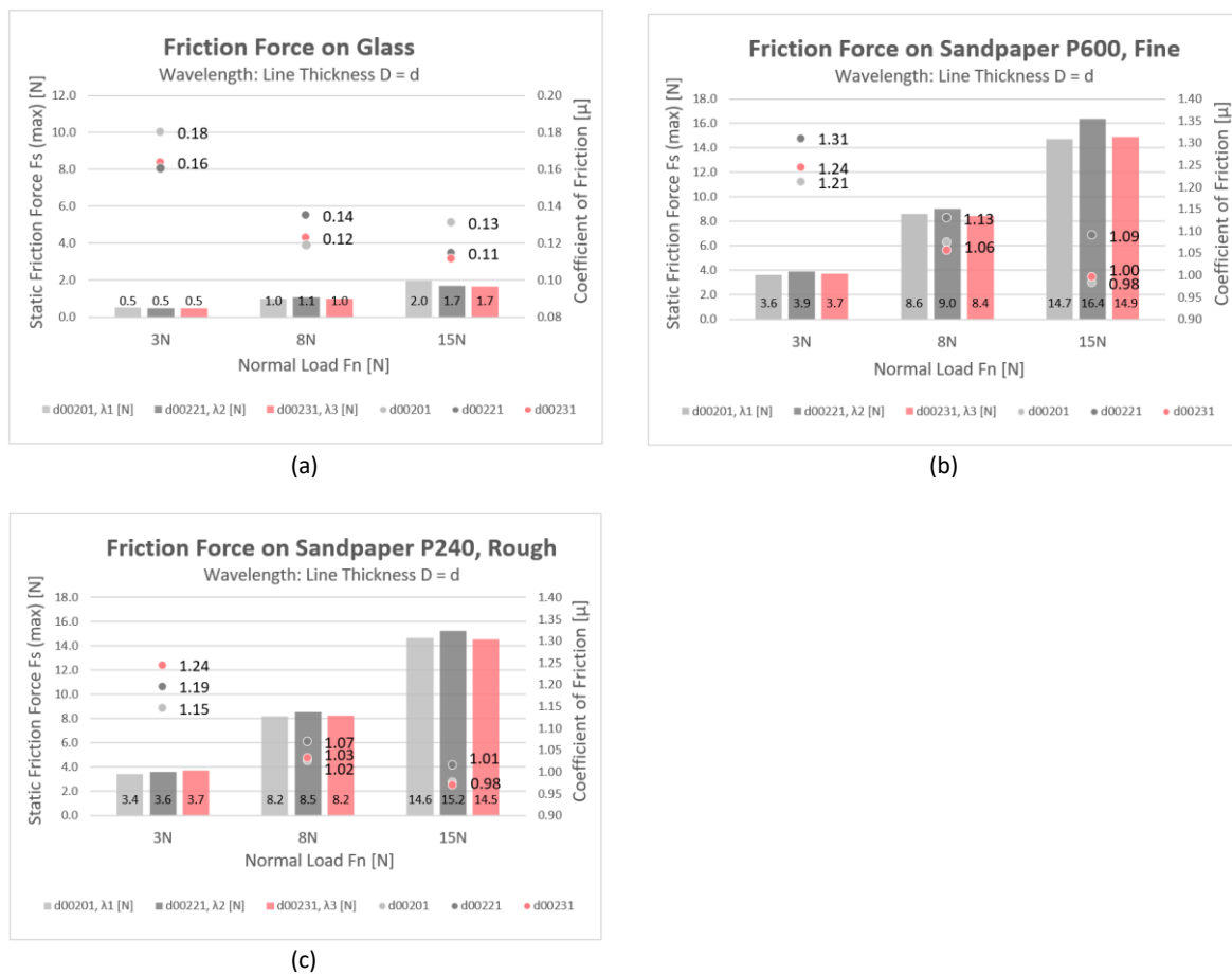
Figure 7.5. The maximum static friction force F_s (max) [N] and coefficient of static friction \mu_s of 3D printed lines, with variable wavelength \lambda_1 = 2.8 mm, \lambda_2 = 1.8 mm and \lambda_3 = 0.8 mm, for the countersurface glass (smooth), sandpaper P600 (fine), and sandpaper P240 (rough). The measured F_s (max) is represented by columns and the corresponding \mu_s is represented by dots.
