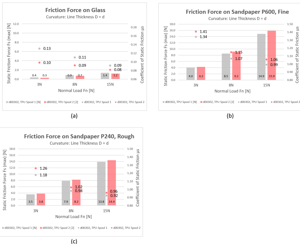
Figure 9.1. The maximum friction force (max.) F_s [N] and coefficient of static friction \mu_s of 3D printed lines, with variable angle \alpha_1 = 0^\circ , \alpha_2 = 68^\circ with an inner radius of 16 mm, and \alpha_3 = 124^\circ with an inner radius of 10 mm, for the countersurface glass (smooth), sandpaper P600 (fine), and sandpaper P240 (rough). The measured F_s (max) is represented by columns and the corresponding \mu_s is represented by dots.
