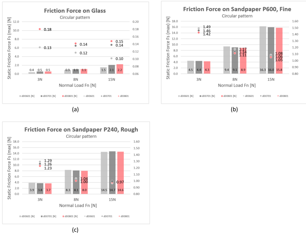
Figure 9.3. The maximum friction force (max.) F_s [N] and coefficient of static friction \mu_s of 3D printed circular patterns with: (a) 68° curvatures and an inner radius of 16 mm (d00601), (b) circular shape as the starting point with an inner diameter of 3.5 mm (d00701), (c) and a combined shape of a square and half a circle with each an inner diameter of 3.5 mm (d00801), for the countersurface glass (smooth), sandpaper P600 (fine), and sandpaper P240 (rough). The measured F_s (max) is represented by columns and the corresponding \mu_s is represented by dots.
