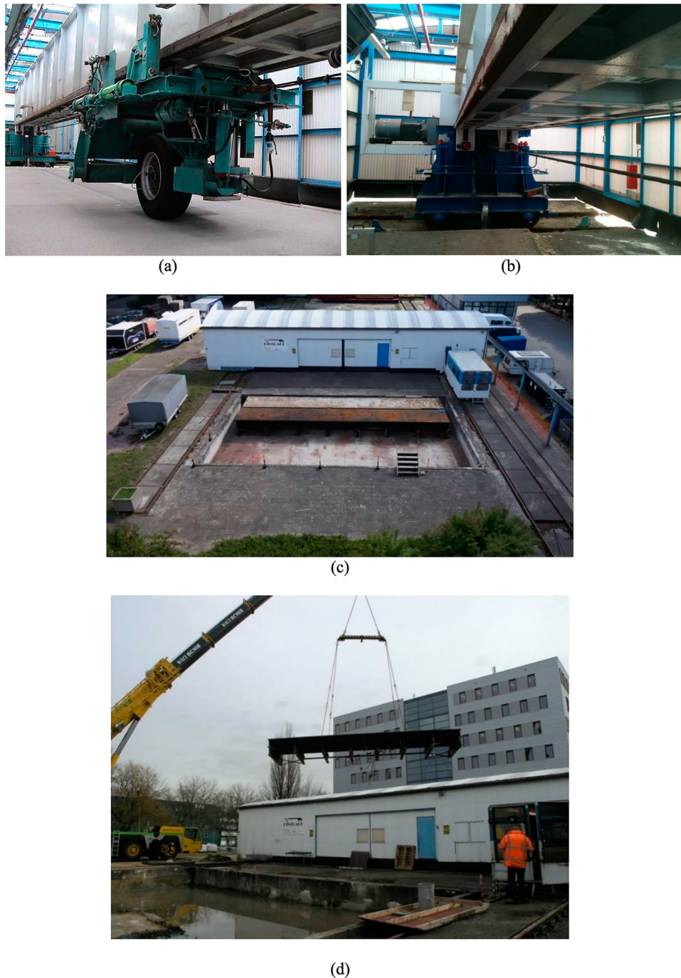
Figure 3. LINTRACK accelerated pavement testing; (a) apparatus, (b) guidance system supports on transverse rails, (c) housing unit, and (d) steel bridge deck placement.
