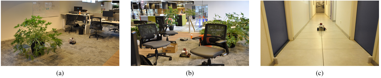
Fig. 3: Indoor test environments used for performance evaluation of FEEL. a) E_1 : office environment with sparsely distributed objects, b) E_2 : office environment with densely distributed objects, and c) E_3 : narrow, long corridor with no other objects.
