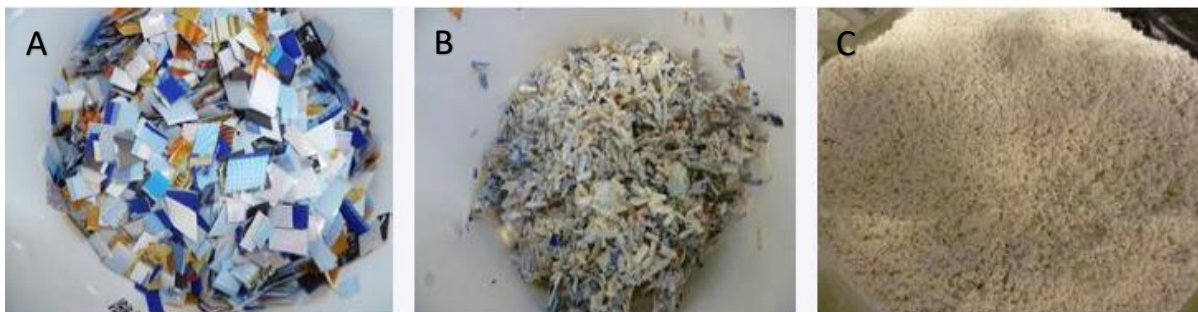
Figure 5: Lab-scale solvent dissolution of (A) three-layer PP/PA/PE film to remove (B) insoluble adhesives, inks and PA layer and recover (C) PP and PE flakes (Roelands, 2021).
