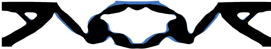
Figure 7.24: A visualization of the difference between the displacement magnitudes of the topologies obtained for global minimization (blue) and local minimization of the input and output area (black) for the excitation frequency \omega_{exc}=471\text{Hz} and \gamma_1=0.90 .
