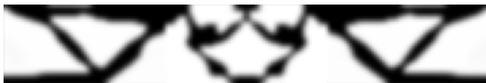
Figure 7.7: The structure obtained when the resulting inverter mechanism and isolator of figure 7.2a and 7.6a respectively are stitched together.
