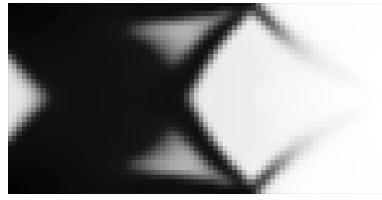
Figure 4.23: The resulting topology from the design problem given in figure 4.21a without additional mass added to the response point.
