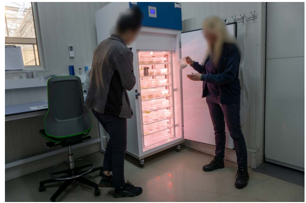
Figure 36.2: Climate cabinet with plastic containers with seeds.
