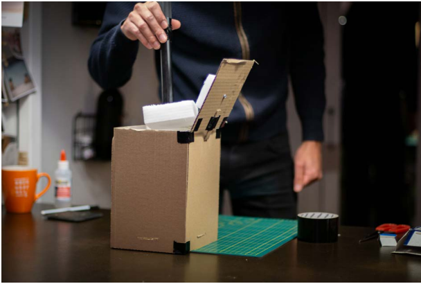
Figure 27.2: User testing seed placing with a mockup of a vacuum seed placer.
