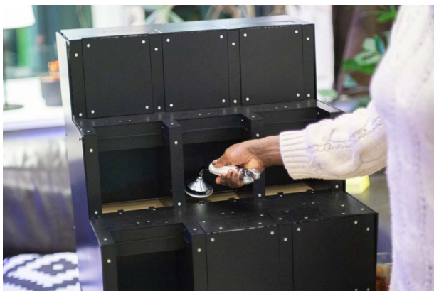
Figure 36.9: User placing seeds with a vacuum head mockup. All cells were opened simultaneously.
