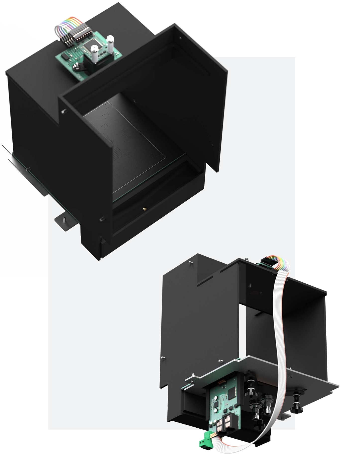
Figure 1.3: The cells have temperature-controlled floor surface, on which filter papers with seeds can be placed to perform germination tests. The control electronics are placed in the bottom of the cell.
