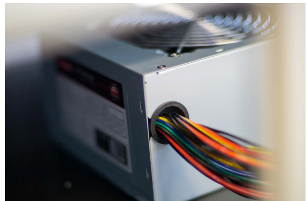
Figure 3.9: Power supply inside the Array.
