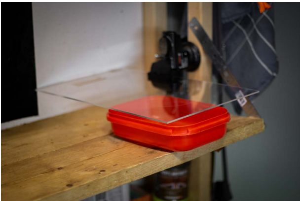
Figure 29.1: The test setup, with an acrylic plate with a hydrophobic foil applied. Here, there was no hot water in the tray.
