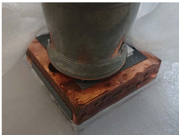
Figure 6.1: Test setup of a Peltier element with temperature control (in Quantified's lab).
