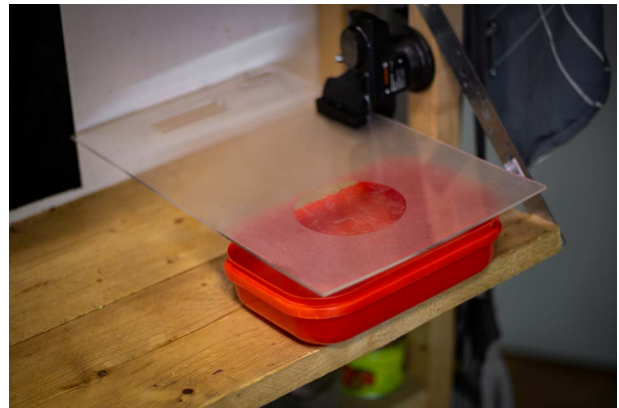
Figure 29.2: The test setup just after the tray is filled with hot water.
