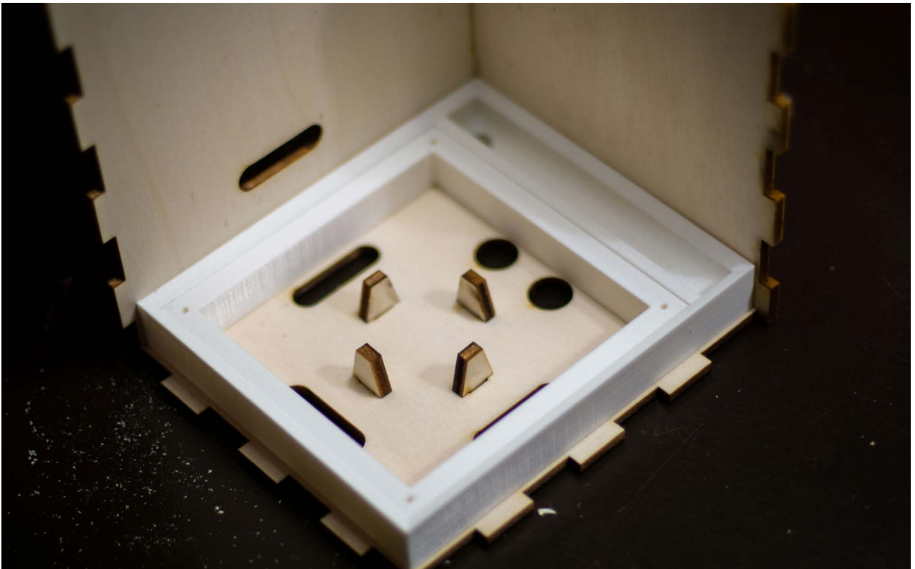
Figure 26.5: Prototype of PCB holder and water drain.
