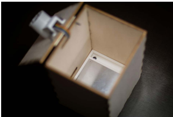
Figure 27.5: The inside of the cell with a PCB holder and PCB, water drain. The camera is also attached.
