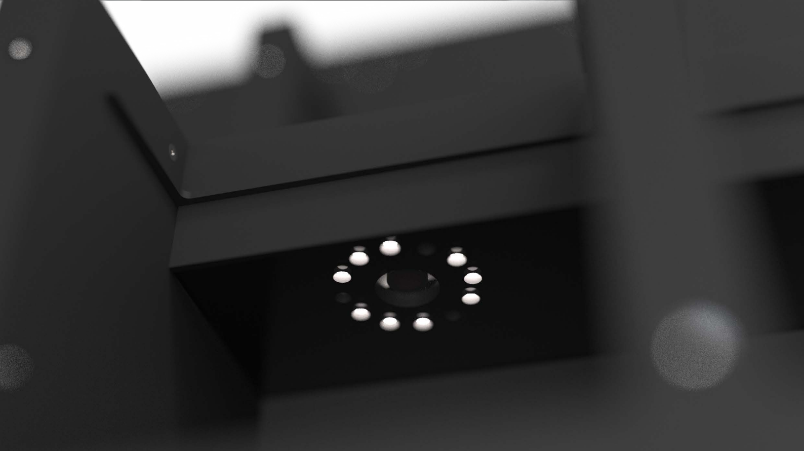
Figure 1.12: A transparent window protects the camera and the surrounding electronics from moisture from within the cell. The LED rings are used to provide light for the seeds and as a camera flash.
