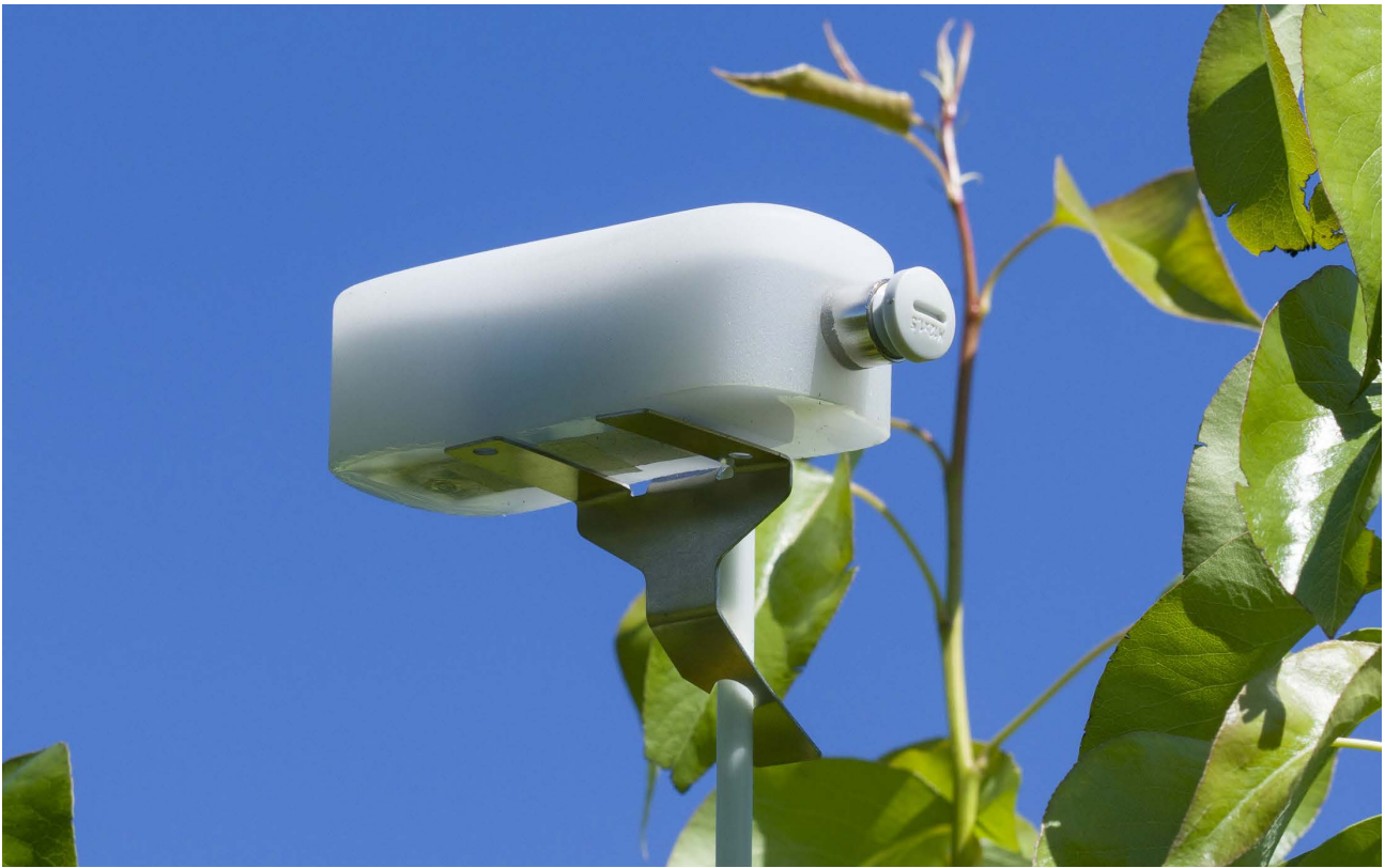
Figure 5.7: Quantified's climate sensor.
