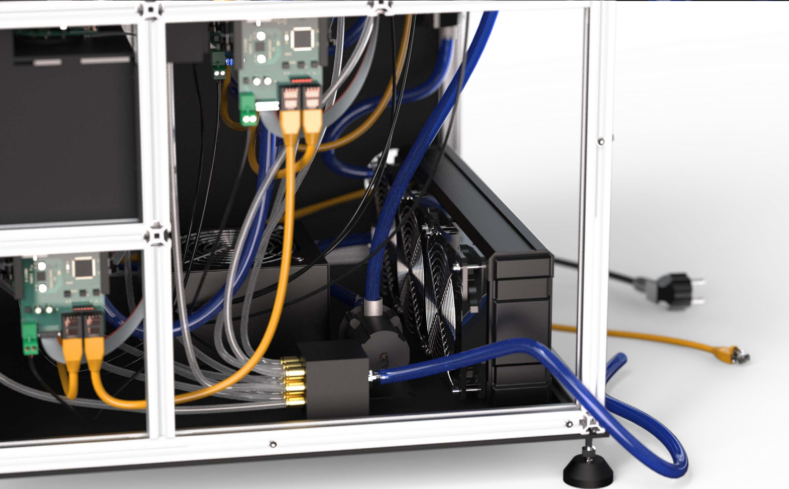
Figure 1.10: The pump, heat exchanger are situated in the bottom of the QIEM-Array.
