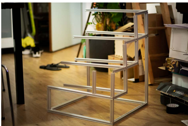
Figure 3.1: Construction of the frame with aluminum extrusion profiles.
