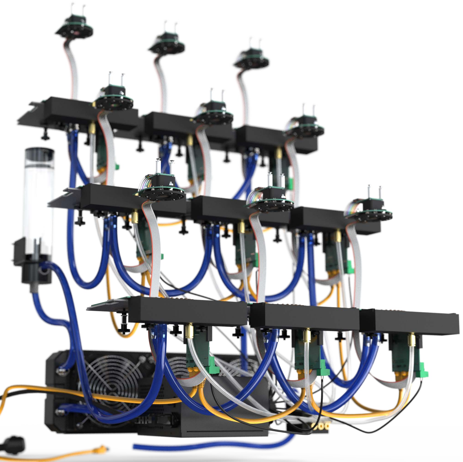
Figure 1.14: The QIEM-Array with some of the walls removed to make the inside connections visible.
