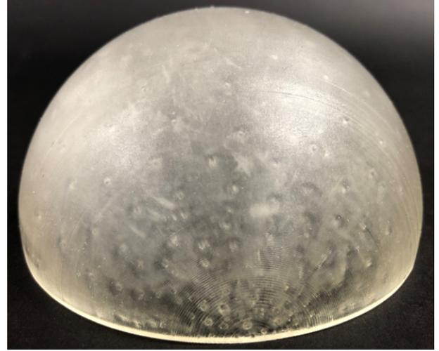
Fig. 16. Hemisphere printed in x/y-direction
