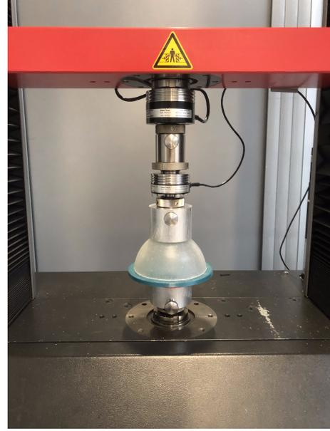
Fig. 4. Test setup unequal surfaces compression
