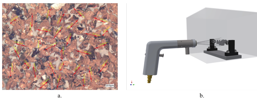
Fig. S1: a) 50 micron Alumina ( Al_2O_3 ) abrasive used for shot blasting. b) Schematic shot blasting setup.
