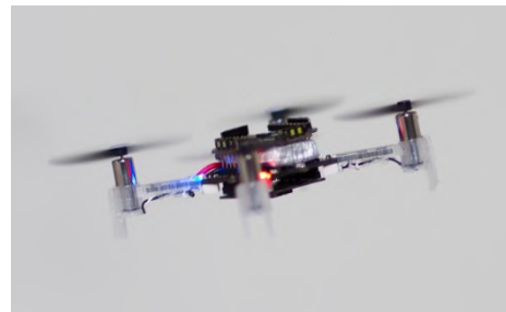
Fig. 9. Crazyflie, a 39-gram MAV from company Bitcraze.
