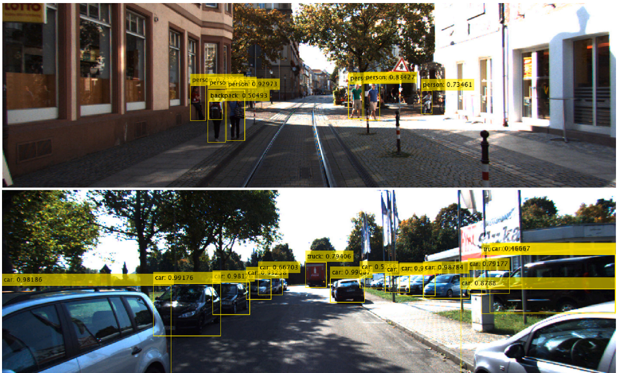
Fig. 2. Results of YOLOv4 for 2 of the 210 images. In the upper image, the algorithm identified six persons and a backpack. In the lower image, the algorithm identified 13 cars and 2 trucks.
