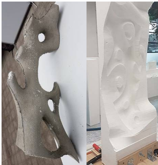
Fig. 3. Top: Real-scale fragment’s multi-layered fabrication / integration logic. Bottom: Robotically fabricated concrete (left) and EPS (right) fragments.
