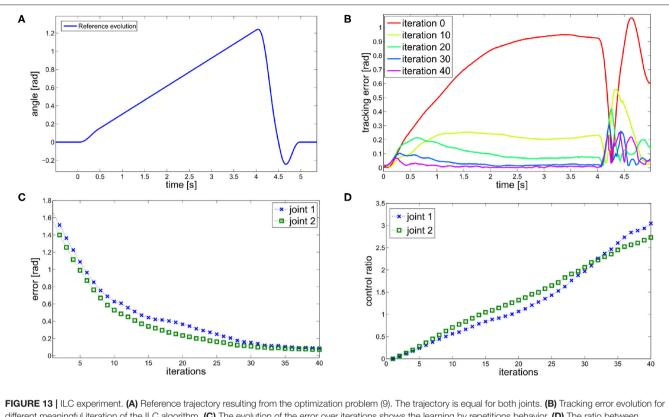
FIGURE 13 | ILC experiment. (A) Reference trajectory resulting from the optimization problem (9). The trajectory is equal for both joints. (B) Tracking error evolution for different meaningful iteration of the ILC algorithm. (C) The evolution of the error over iterations shows the learning by repetitions behavior. (D) The ratio between feedforward and feedback actions shows an anticipatory behavior.
