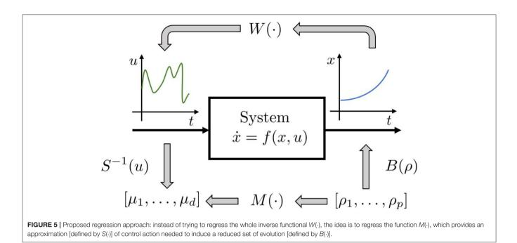
Several approaches can be applied to compute the inverse functional *W*. Some methods contemplate the independent estimation of a complete model of the system (e.g., Arif et al., 2001; Purwin and D'Andrea, 2009). The limitations of complete model estimation (Nguyen-Tuong et al., 2008) approaches are well-known (e.g., computational onerous). Conversely, in our approach we will focus on a reduced space of control actions and trajectories, in order to limit the computational burden.
