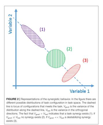
(performance) variable." Given an "important output variable" we can define two variables  $V_{good}$  and  $V_{bad}$ .  $V_{good}$  is the variance through the directions where output is constant and the constraints are verified (named *uncontrolled manifold*), while  $V_{bad}$  is the variance in the other directions (Scholz and Schöner, 1999). The system presents a synergistic behavior when  $V_{good} > V_{bad}$ . Figure 2 visually explains this point.
