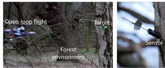
Figure 1.5: Drone placing a sensor in a forest environment [11]
