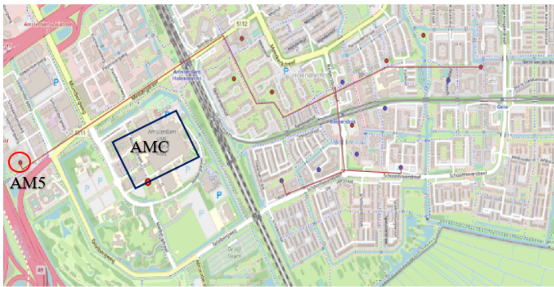
Figure 3.4: The DHN network backbone mapped on the QGIS software
