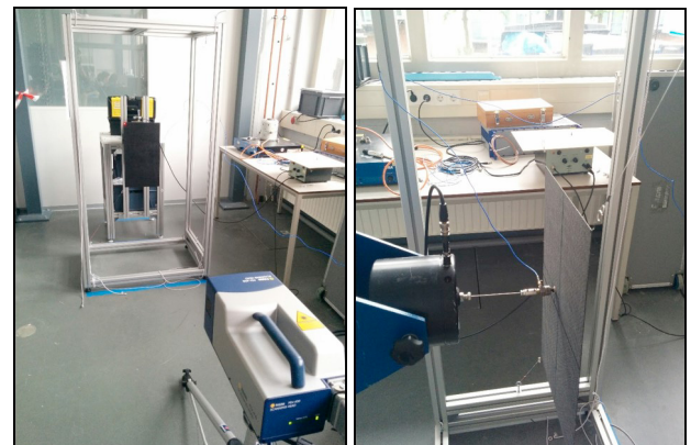
(a) Laser Doppler Vibrometer (b) Shaker and impedance setup
