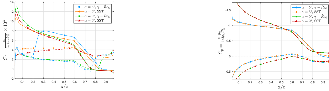
Figure 7: Skin friction (left) and pressure (right) distributions for both AoA. Both SST and \gamma - \tilde{Re}_{\theta_t} , ( [I, \frac{v_t}{v}] = 1 ) results are shown.
