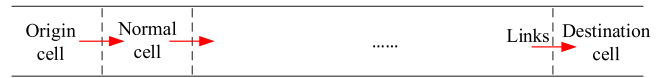
Fig. 1. The depiction of cells and links. Red arrows represent links, and black dashed lines represent the boundaries between cells. Origin cells have no incoming link and destination cells have no outgoing link. Normal cells are connected by one incoming link and one outgoing link.
