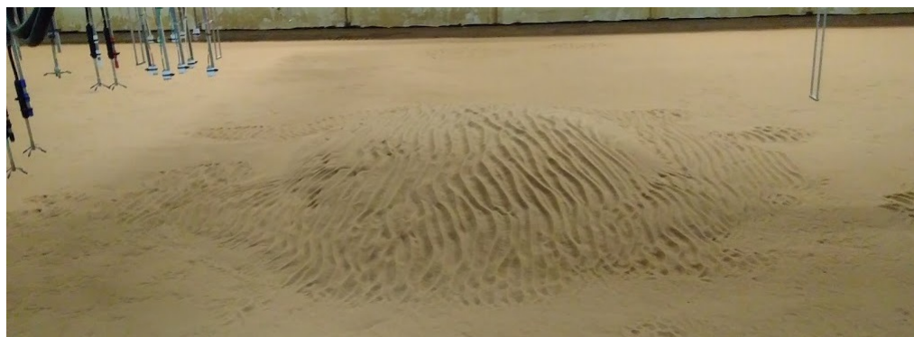
Figure 4.3: Mound morphology after the end of scenario 1 (low waves). The flow direction is from right to left.
