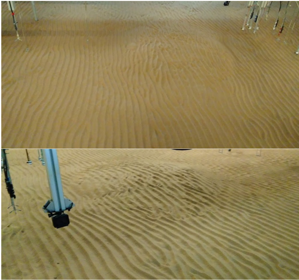
Figure B.12: Top: Mound morphology after the end of scenario 3. Top: The focus is at the front of the mound. The flow direction is from left to right. Bottom: The focus is at the back of the mound. The flow direction is from right to left.
