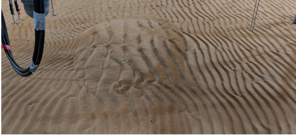
Figure B.24: Top: Mound morphology after the end of scenario 8 (combined, more current). The flow direction is from left to right.
