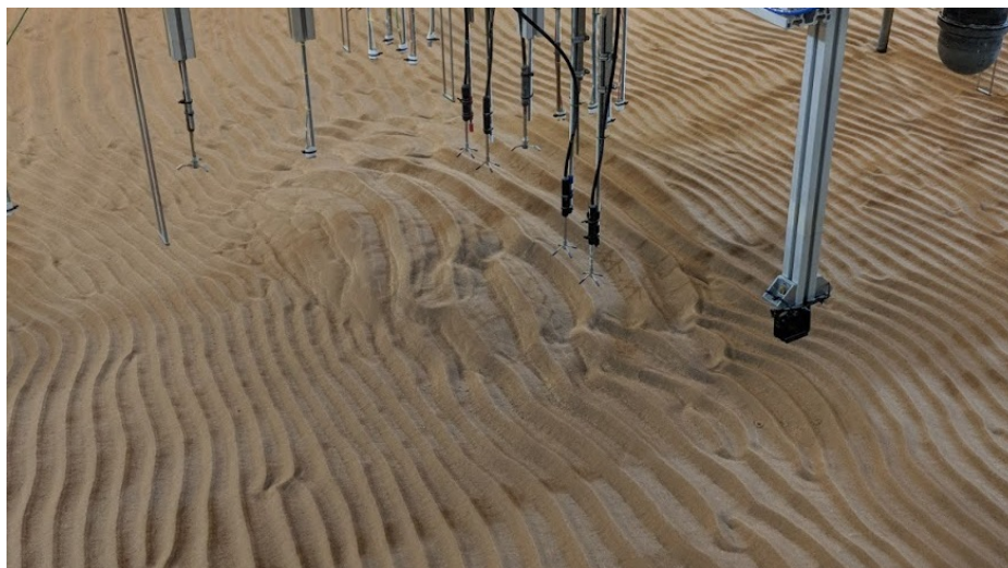
Figure 4.11: Mound morphology after the end of scenario 7 (combined, equal contributions). The flow direction is from right to left.
