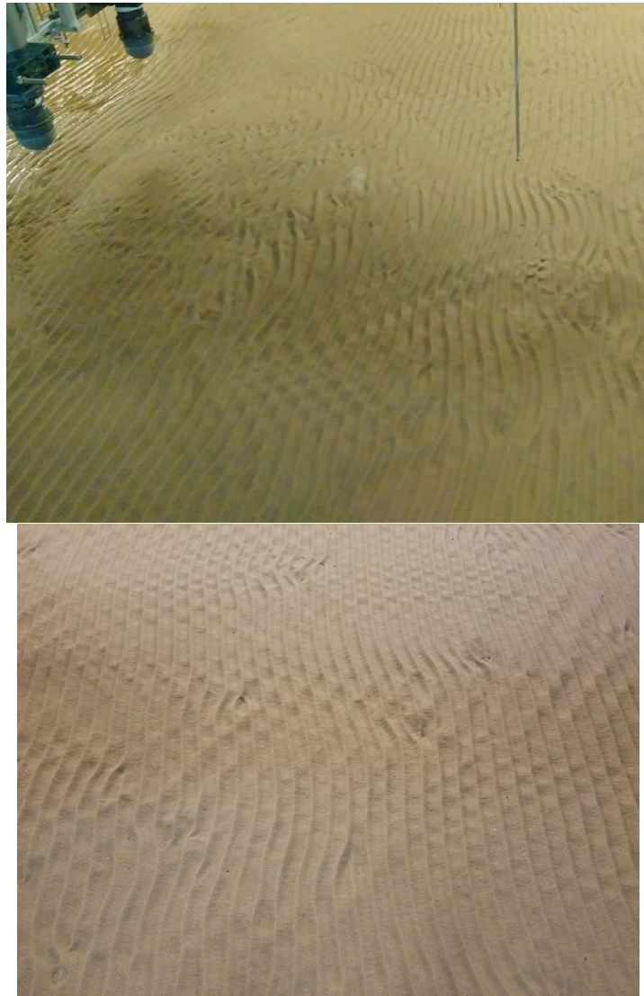
Figure B.5: Top: Mound morphology after the end of scenario 2. The flow direction is from right to left. Bottom: Ripple checked pattern after scenario 2.
