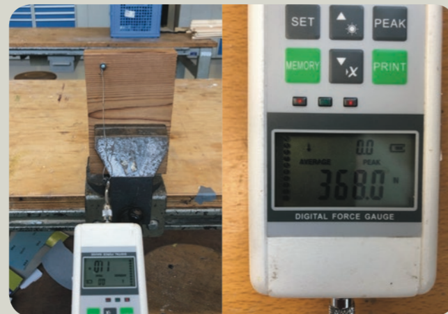
Image 76: Testing the strength of the screw connection. Source: Author.
