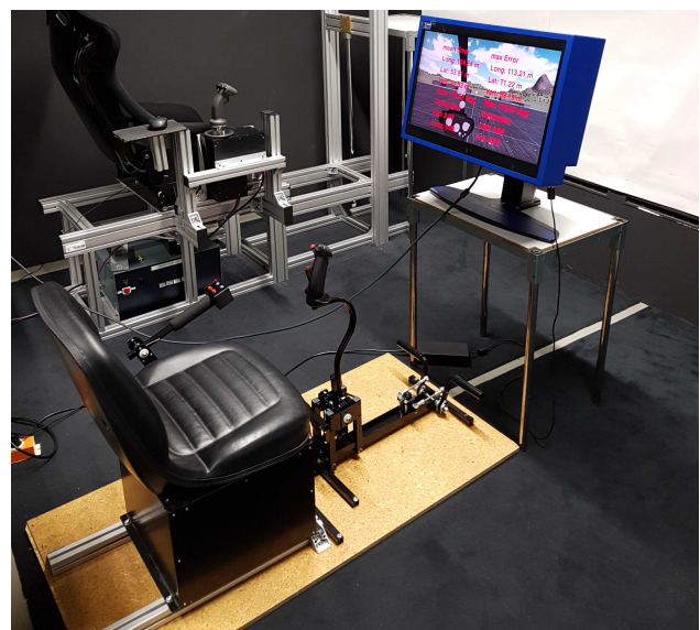
Figure 2: The Computer Based Trainer set-up used in this experiment, equipped with the Pro Flight Trainer ® PUMA helicopter control inceptor.
