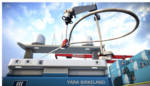
Figure 2.10: Mooring rope with a robotic arm [48]
