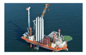
Figure 1.3: Bold Tern from Fred. Olsen Wind Carrier (jack-up vessel) with single components (Fred. Olsen Windcarrier).
