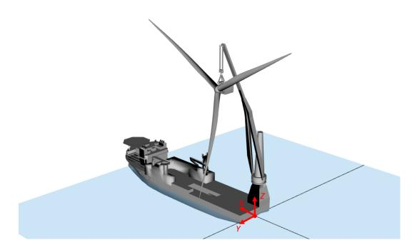
Figure 6.1: Overview of *Model 3 - Wind & Waves*. The global coordinate system is shown as well, which has its origin at MSL, stern, centerline of the vessel.
