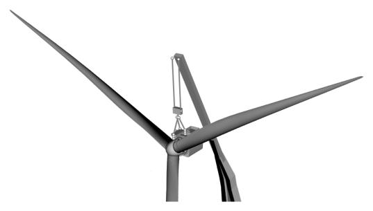
Figure 2.5: Rigging arrangement for installing the RNA using three slings from crane block to lift frame. The lift frame is rigidly connected to the RNA. The nacelle is modelled as one body and the rotor as another body that is rigidly connected to the nacelle
