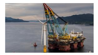
Figure 1.5: Saipem 7000 from Saipem S.p.A. (semi-submersible) installing the Hywind, a floating wind turbine (Timperley, 2017).
