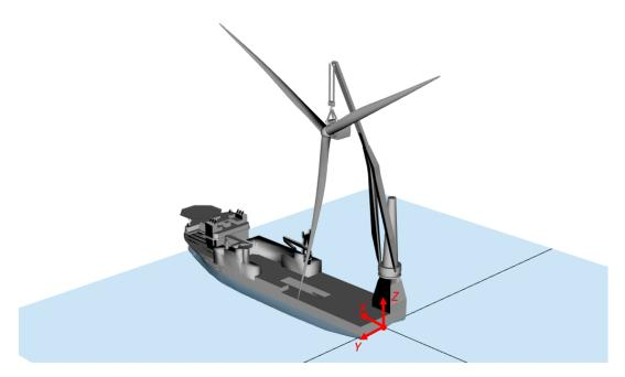
Figure 7.1: Overview of *Model 3 - Wind & Waves*. The global coordinate system is shown as well, which has its origin at MSL, stern, centerline of the vessel.
