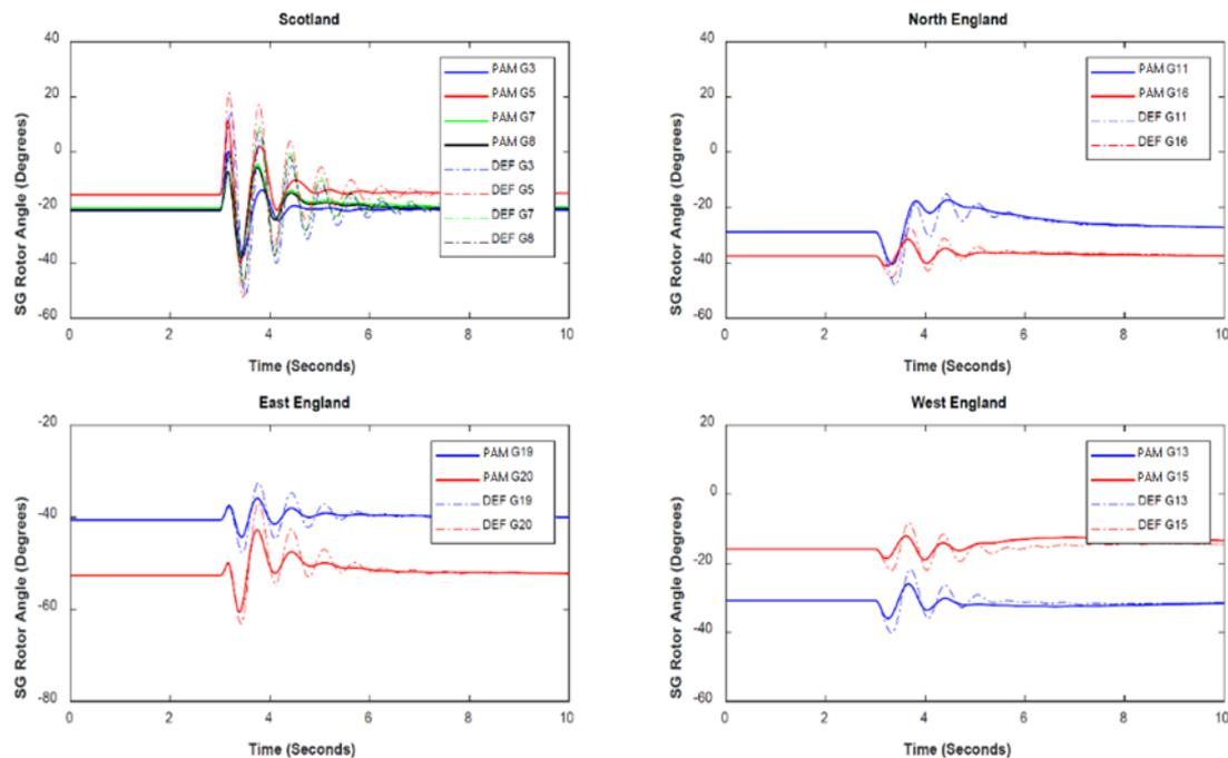
**Figure 14.** SGs' rotor angles responses for a 120 ms three-phase fault at Line 6–9 under a 66% share of wind generation in the GB system. Solid lines—WGs with PAM controller enabled, dashed lines—WGs without PAM controller enabled, default (DEF) response.
