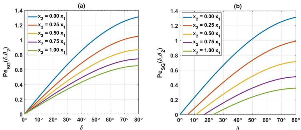
**Figure 2.** The power-angle curves of the synchronous generator SG1 are exhibited under different  $x_1$  and  $x_2$  ratios: (a) the active power provided by the WG1 unit is null, (b) the active power provided by the wind generator WG1 unit has been increased to 50% of the SG1 rated power.
