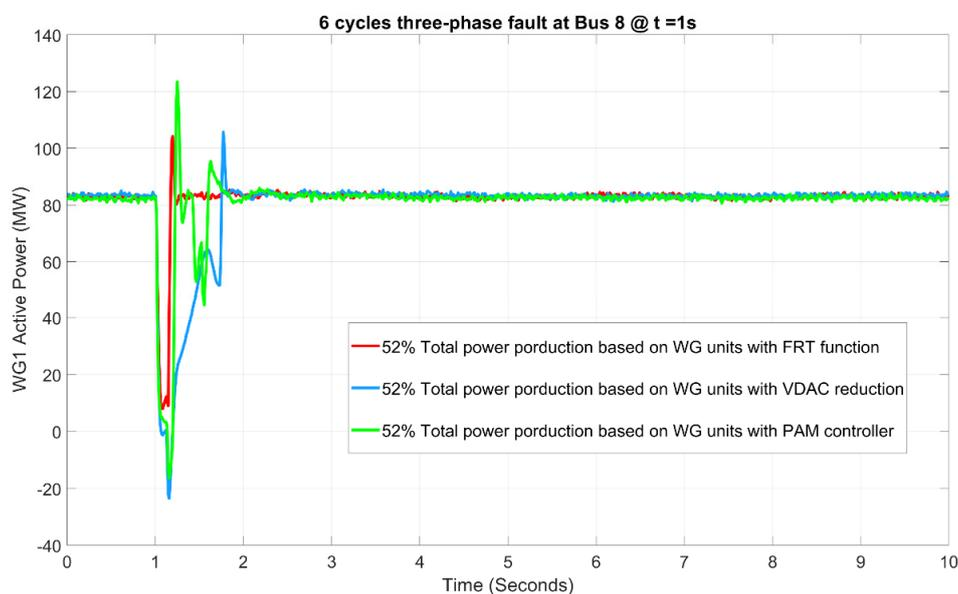
**Figure 11.** The active power deployments produced by the FRT function (red), the voltage-dependent active current (VDAC) reduction (blue) and the PAM controller (green) under a large disturbance event occurring at BUS 8.
