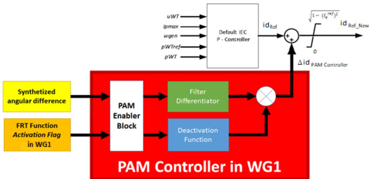
Figure 6. Basic structure of the PAM controller.
