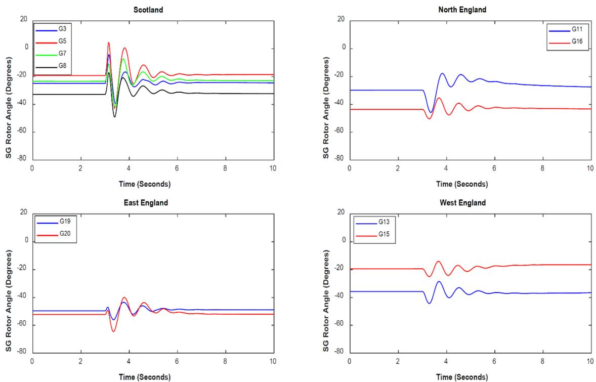
**Figure 16.** SGs’ rotor angles responses for a 120 ms three-phase fault at line 6–9 under a 66% share of wind generation in the GB system. WGs with the PAM controller only activated in Scotland and the East England areas of Figure 13.
