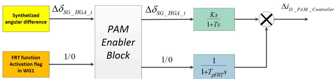
**Figure 7.** Internal control scheme of the PAM controller altering the active current modulation (during and after the fault period) based on the fault ride-through (FRT) function activation in the WG unit.
