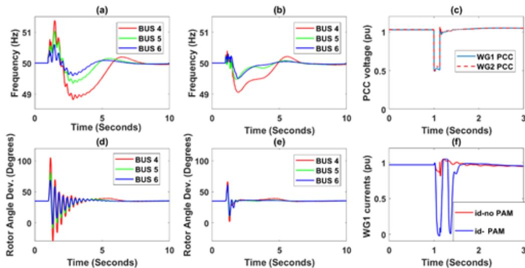
**Figure 10.** Faults implemented far from the wind turbines (a) frequency response without PAM connected, (b) frequency response with PAM connected, (c) voltage drop in the WGs PCC voltages for BUS 5 fault, (d) rotor angle deviations without PAM, (e) rotor angle deviations with PAM, (f) WG1 currents after BUS 5 fault.
