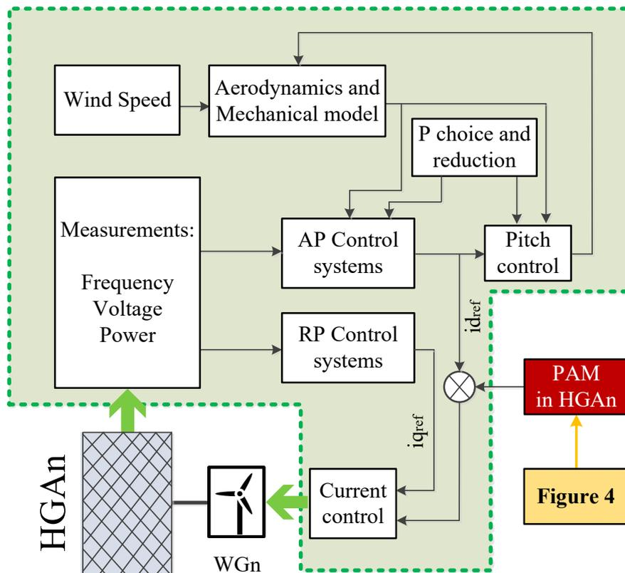
**Figure 5.** Control layout of the WG power plant located in the hybrid generation area n (HGAn) based on the The International Electrotechnical Commission (IEC) 61400-27-1 international standard (green box) in which the PAM controller has been included for modification of the WGn active ( $i_{dref}$ ) current.
