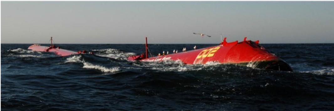
Figure 2.2: The PELAMIS wave energy converter. Image has been taken from Yemm [17].
