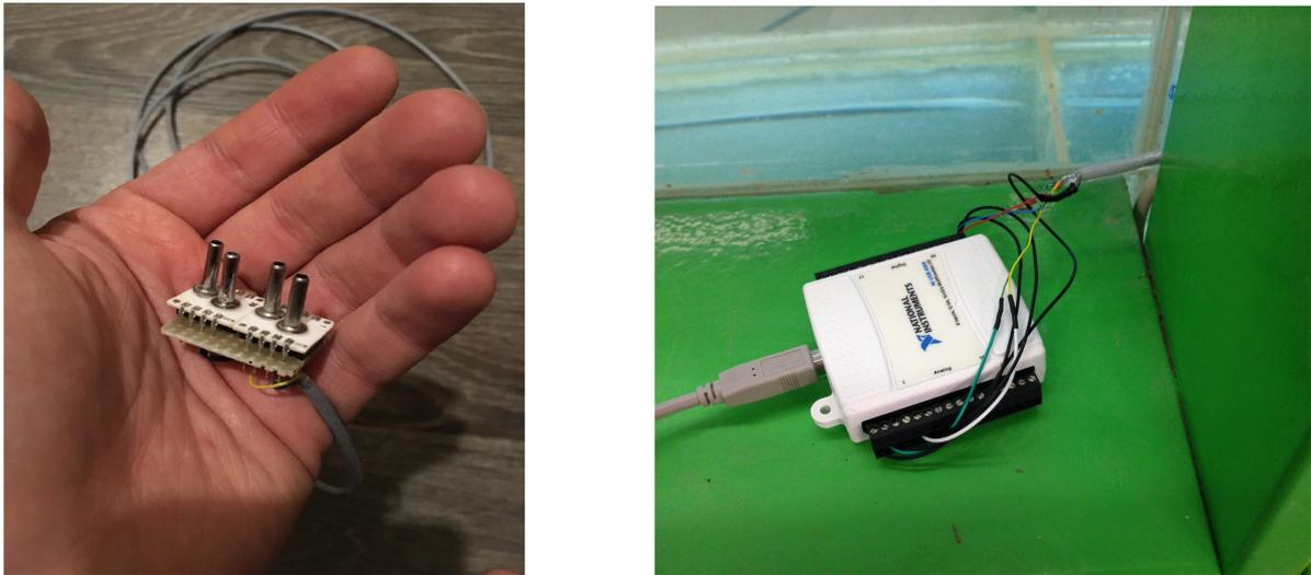
Figure 5.11: Pressure sensor and the interface device used for the data acquisition. Each sensor contains two cylinders to measure the difference in pressure between them. One of these is connected to the atmosphere while the other measures the air pressure in the chamber.
