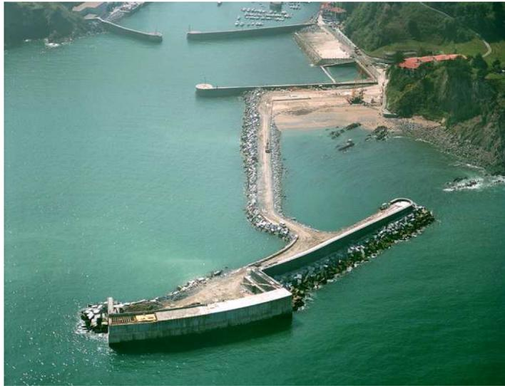
Figure 2.1: The Mutriku breakwater oscillating water column from the air. This image has been taken from Marqués et al. [9].
