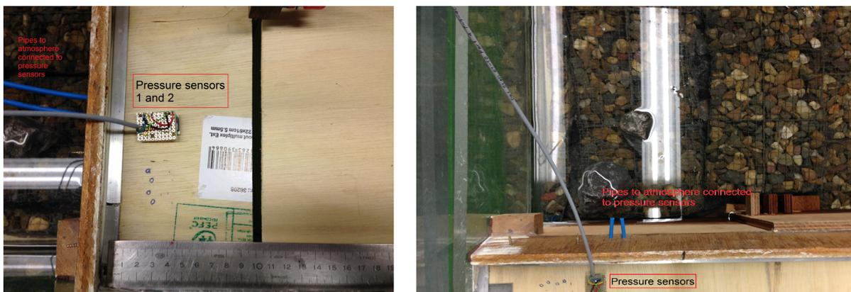
Figure 5.10: Pressure sensor on the damping lid of the system.
