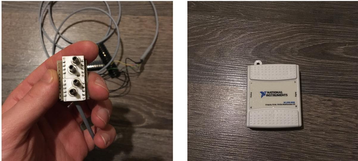
Figure C.2: Pressure sensor and interface device.
