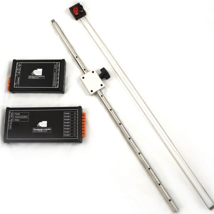
Figure C.1: Wave gauge and controller. This image has been taken from [48].
